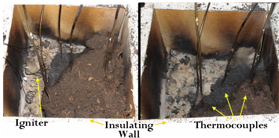
Figure 4. Two snapshots during one of the experiments that reached strong ignition of the peat (moisture content 100%) showing the progression of the smouldering front. Location of the igniter and the thermocouples is indicated. Time elapsed between the left and the right photographs is about 1 h. Note that propagation is not uniform across the box.
