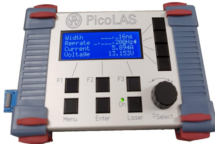
Figure 4.9. PLB-21 controller unit that can be calibrated to the specific LD in use and allows the user to independently control the pulse length, rep rate and current. The LED indicator on the unit shows when the LD is active.
