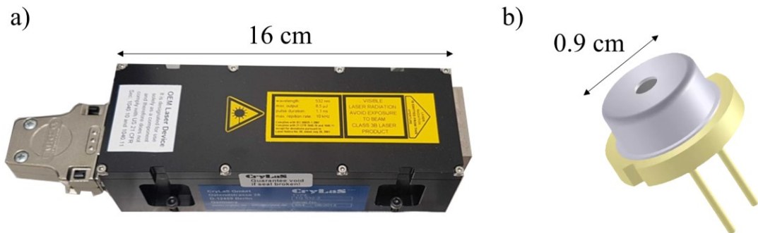
Figure 4.7. Pump lasers used throughout this work with a) the 532 nm Q-switched laser being more than ten times larger than b) the 445 nm laser diode [128].
