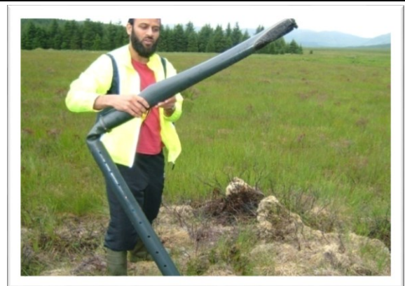
D: water level recorders were severely damaged
