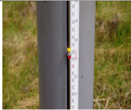
B: The Yellow and Red markers showed here at set to the current water table position
