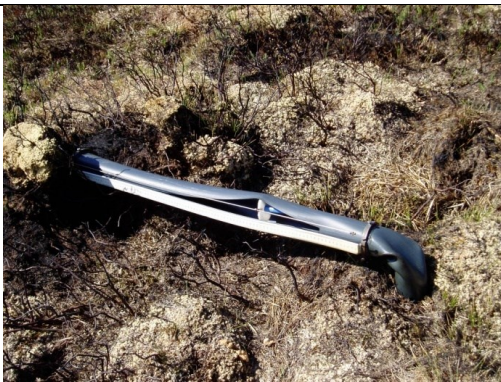
C: Fire damaged the Water level recorders
