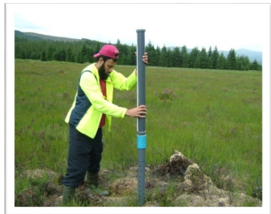
F: Replacing the damaged one with the new recorders
