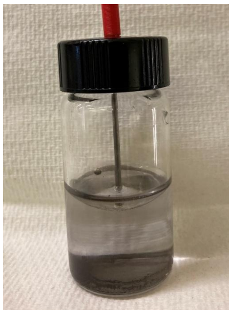
Figure 3.2. Image of screw-top borosilicate glass vial, containing 1%wt nucleating agent (on the bottom), 10 ml of ultra-pure, filtered water, and 1 ml layer of silicone oil on the top, into which sits the thermocouple.
