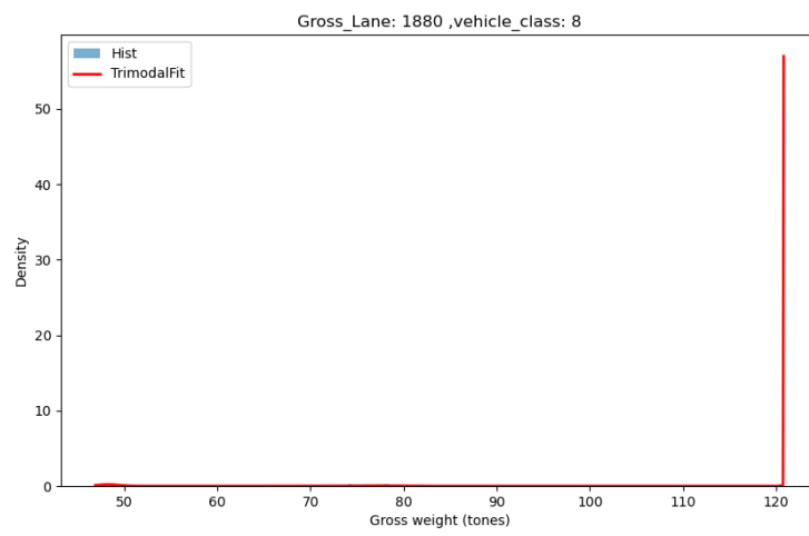
Figure A.25: Gross weight trimodal distribution for class 8 on lane 1880
