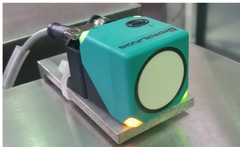
(c) Displacement Transducer ( 6\text{cm} \times 4\text{cm} )
