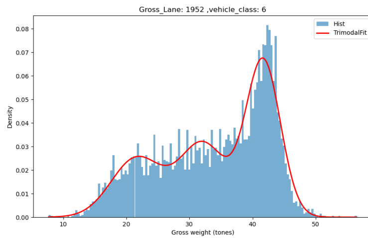
Figure A.17: Gross weight trimodal distribution for class 6 on lane 1952
