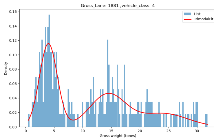
Figure A.9: Gross weight trimodal distribution for class 4 on lane 1881
