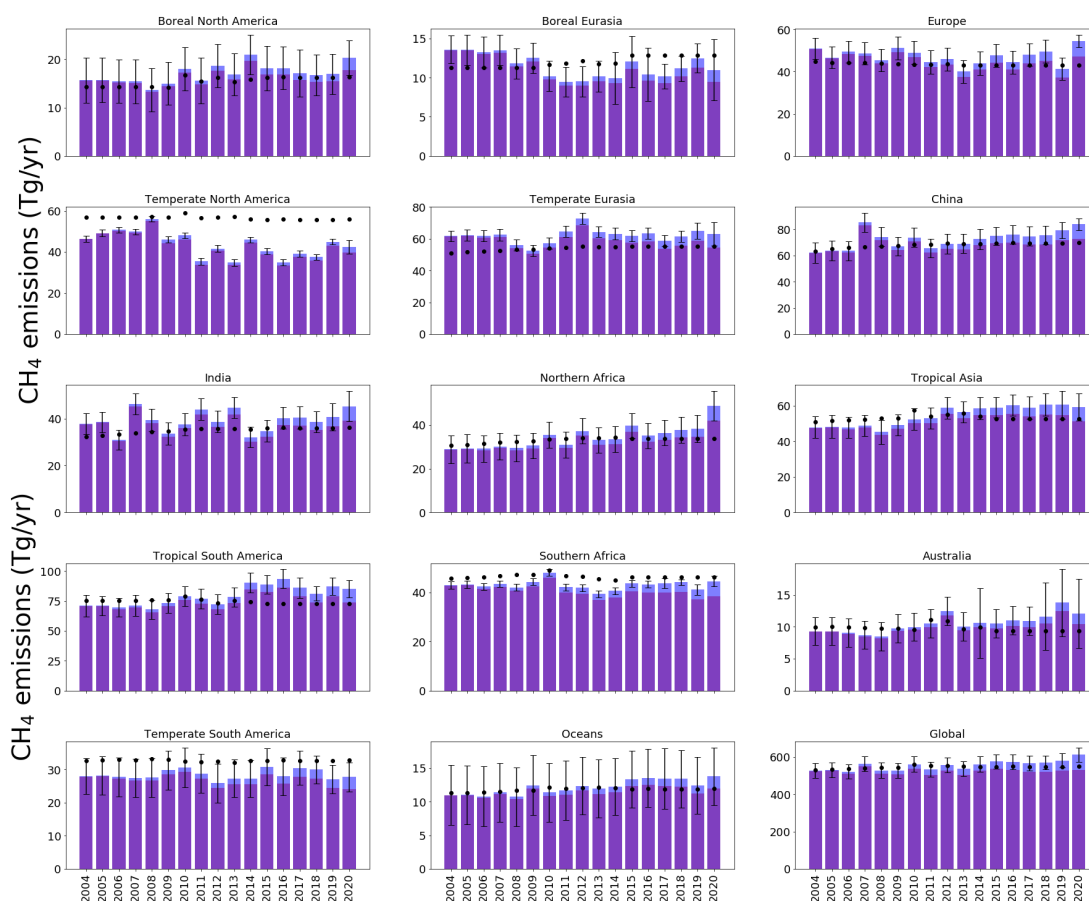
Figure 2.15: Comparing yearly emissions (Tg/yr) for each region of the inversion (indicated by Figure 2.1), for the a posteriori CH 4 simulation (using ground-based data; blue) and the regional emissions of the OH tests (as described in-text; red). OH tests always result in lower emissions than a posteriori emissions. Regional uncertainties for the a posteriori emissions are indicated.
