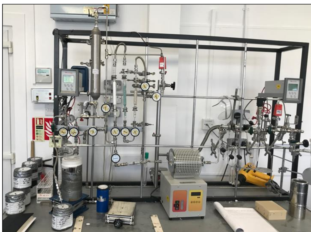
Figure 2-3: Gas combustion line at SUERC, which was used for methane and CO 2 gas stable isotope analysis. Photo shows the Glasgow UKGEOS Isojars connected directly to the extraction inlet for the line.
