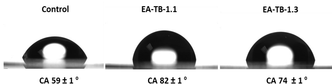
Figure 6.11. The water contact angle measurements performed on the glass coverslips coated with the polymers EA-TB-1.1 and EA-TB-1.3. The control was an oxygen plasma treated glass coverslip.
