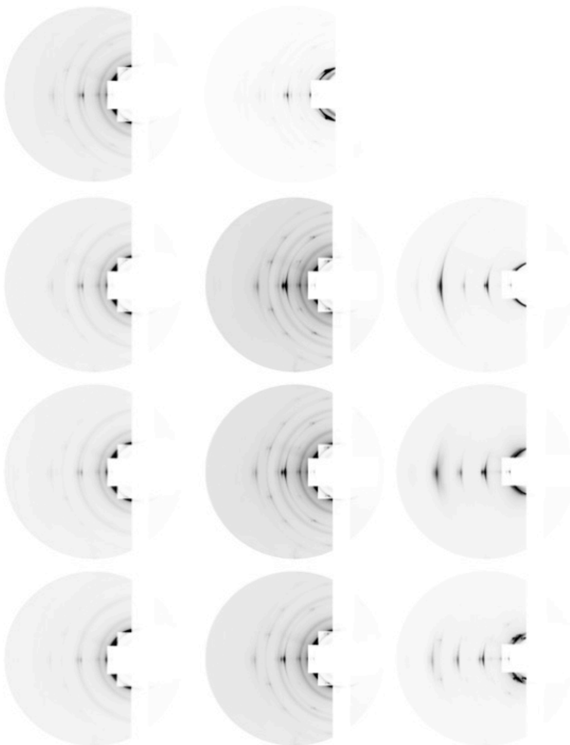
Figure 3.12: Lamellar X-ray diffraction patterns of cis/trans PE samples at different relative humidities (rh). Starting from the top row, 32 °C at 64rh, 66rh, 69rh, 72rh (left to right top row), (middle row) 75rh, 78rh, 81rh, 84rh, (bottom row) 87rh, 90rh, 93rh.
