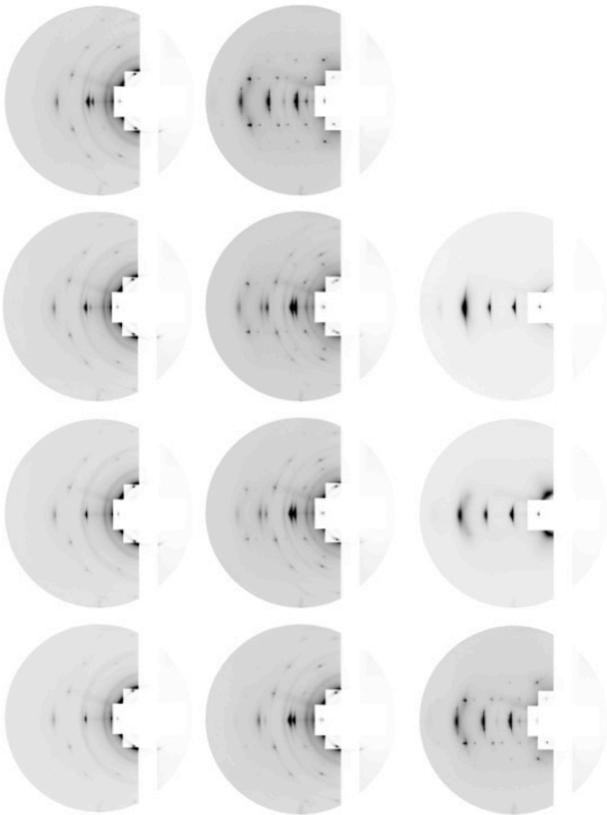
Figure 3.13: Lamellar X-ray diffraction patterns of LS3/DOPE 1 to 100 samples at different relative humidities (rh). Starting from the top row, 32 °C at 64%rh, 66%rh, 69%rh, 72%rh (left to right top row), (middle row) 75%rh, 78%rh, 81%rh, 84%rh, (bottom row) 87%rh, 90%rh, 93%rh.
