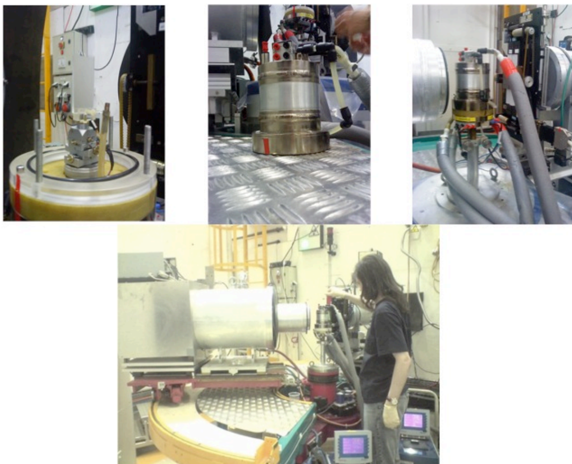
Figure 4.1: The images show the main components in the D16 set-up. The far left image shows the slide with airbrushed sample held on a goniometer and facing the incident neutron beam; underneath the sample is a reservoir of 8% or 25% ^2\text{H}_2\text{O} . The upper middle image shows the sample can unattached. The far right image shows the attached sample can to the rotating sample stage, the attached pipes are connected to two water baths that can adjust the temperature of the water flowing in and out of the can which can create a temperature difference between the bottom and top of the can (the temperature change between the top of the can from the bottom of the can creates the difference in humidity in the sample container, so that even with a temperature change of 1^\circ\text{C} between the top and bottom of the can, there can be a decrease in the relative humidity by 2%). The final image shows the complete set-up of the sample at D16 at the Institut Laue-Langevin (ILL), Grenoble.
