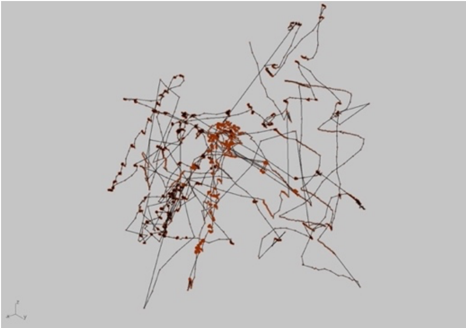
Figure 20: A screenshot from Rhino 3D's viewport while developing the eye-tracked data in the form of a point cloud (in red) into a drawing (black lines) using Grasshopper .
