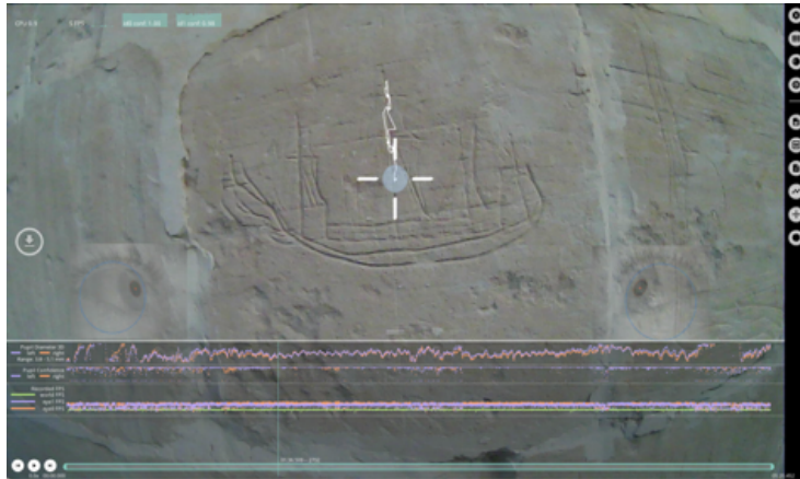
Figure 46: A screenshot of the captured footage by the Pupil Capture binocular device. The screenshot shows my gaze path (in white) as I tried to retrace one of the ship graffiti. It was exported via Pupil Player during postprocessing.
