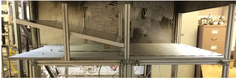
(a) Side view of the experimental set-up with the roofing membrane and wood crib installed in correspondence with the sectional top view in Figure 3.10b.
