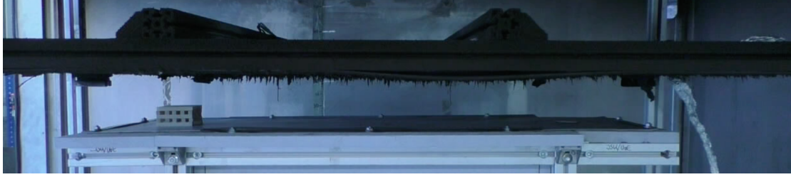
Figure 3.2: Soot buildup below the stainless-steel board due to inadequate cleaning between experiments. Video frame from initial experiments from the MEng thesis of Benjamin Jacobs [5]
