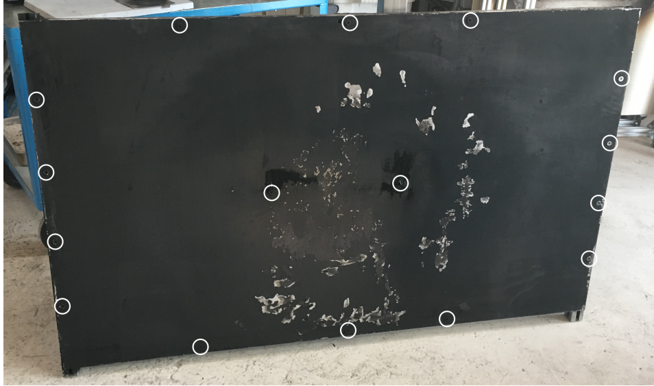
Figure 3.1: Paint damages at the stainless-steel board when brushed down after experiments. The lowered screws are visible on the right side of the board and are marked by white circles.
