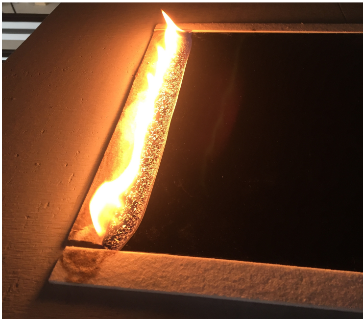
Figure 3.6: Flame front after ignition of a PMMA sample with a sample width of 400 mm.
