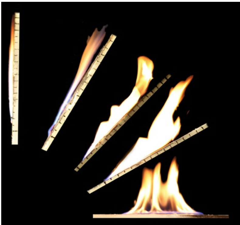
Figure 1.10: Upward flame spread on thermally thick polymethyl methacrylate (PMMA) for surface orientations of 0°, 22.5°, 45°, 67.5°, and 90°. Section of the 2011 IAFFS photo competition winning image by Gollner, Huang, Williams, and Rangwala. [124]
