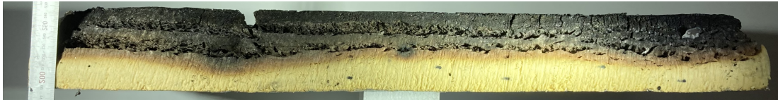
Figure 4.23: Post experiment sectional view along the centre-line for an experiment conducted with PIR insulation and a gap height of 11 cm to a horizontal PV module type 2 (B23 in Table 3.6). The thickness was 80 mm, and the image was mirrored horizontally to ensure a consistent flame spread direction from right to left.
