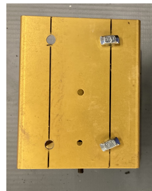
(b) Top view of modified laboratory jack. Two T-bolts installed at the right side.
