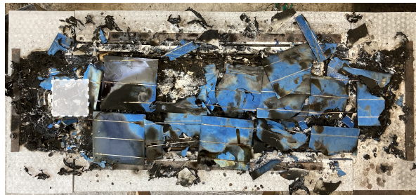
(b) Top view of roof mock-up. The shaded white square with the dotted line marks the location of the wood crib used for ignition. The scattered blue pieces are the non-combustible mono- or poly-crystalline cells delaminated from the PV module.
