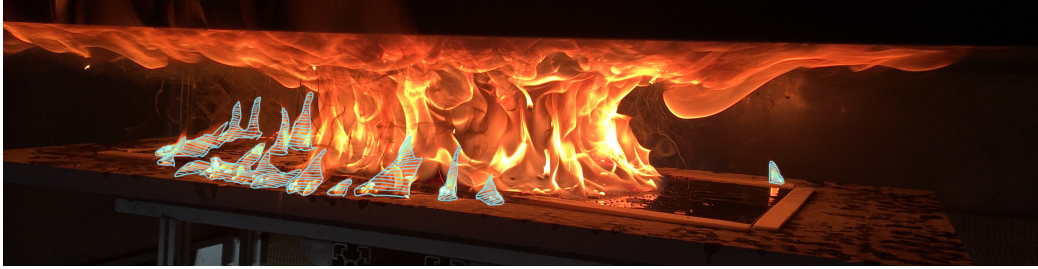
Figure 4.14: Experiment conducted with PV module, sample width of 30 cm, and a gap height of 17 cm. The highlighted flames were molten plastic from the back of the PV module, which continued burning. (From Kristensen et al. [6])
