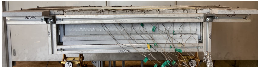
(b) Thermocouples (TCs) installed through a single board of 22 mm thick calcium silicate. The board and the TCs were locked in place by an aluminium profile.
