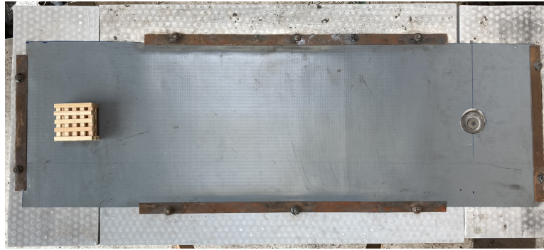
Figure 3.8: Top view of the mock-up roof construction before ignition of the wood crib. The membrane was fastened along the edges to prevent shrinkage, and the four metal rulers were attached to the below aluminium profiles.
