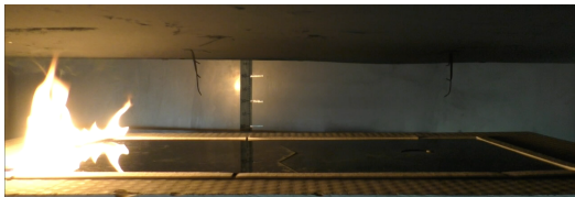
(a) Auto exposure: ON - 10 min after ignition.
