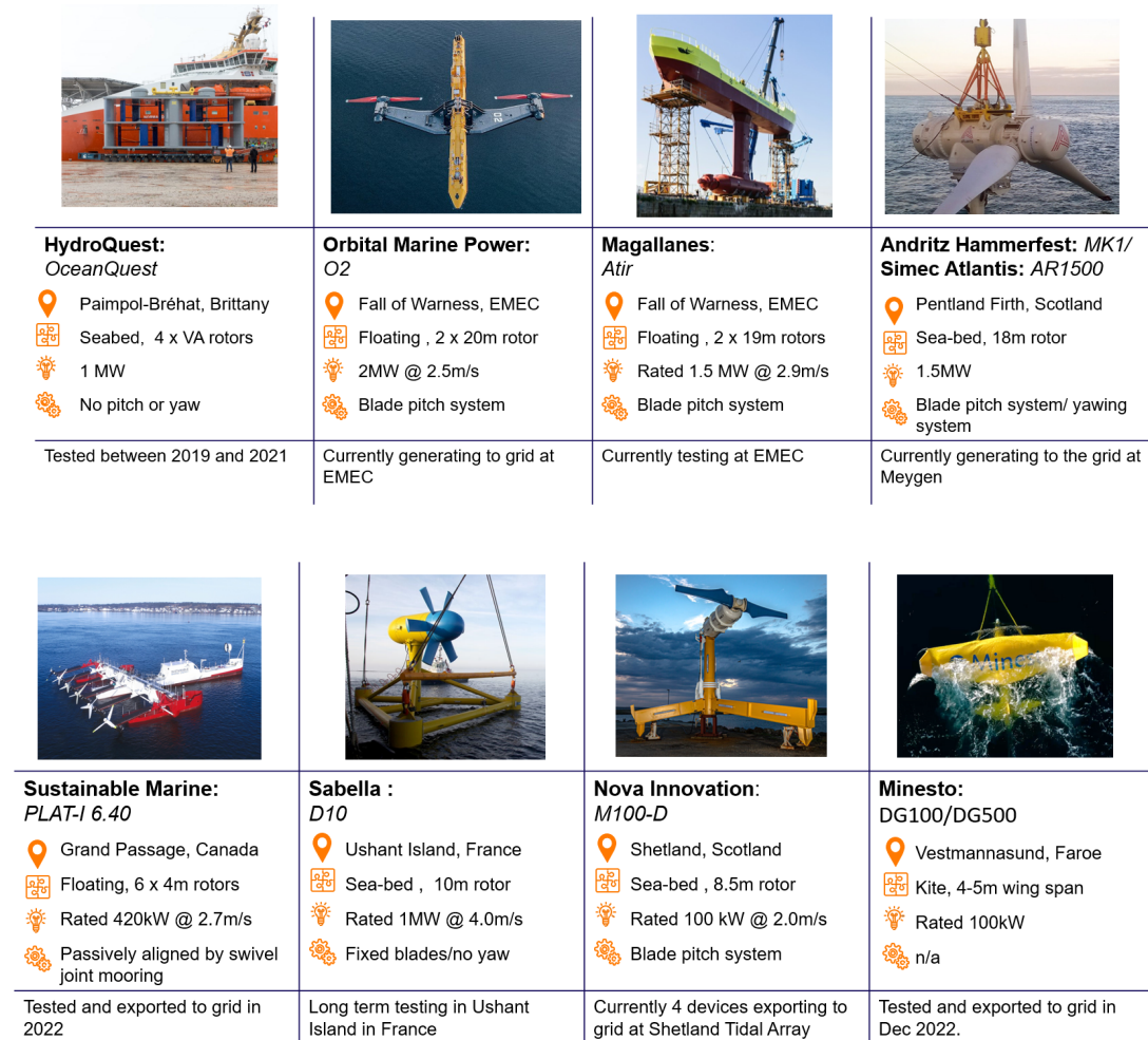
Figure 1.1: Summary of key tidal stream energy developers and their status as at July 2023. HydroQuest (2021), Orbital (2022b), Magallanes (2021), SimecAtlantis (2022), SME (2022), Sabella (2022), Nova (2020), Minesto (2021).
