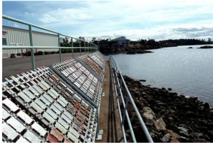
Figure 1-6 Metal samples left at marine environments for corrosion testing 20
