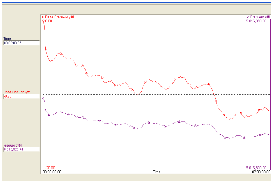
Figure 2-10 Frequency(purple) and change in frequency(red) versus time for Au plated RQCM crystal immersed in deionised water
