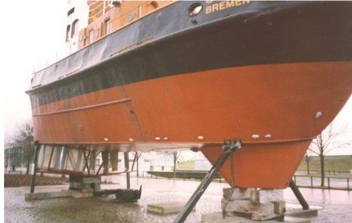
Figure 1-8 Sacrificial zinc anodes attached to the hull of a tug boat 45
