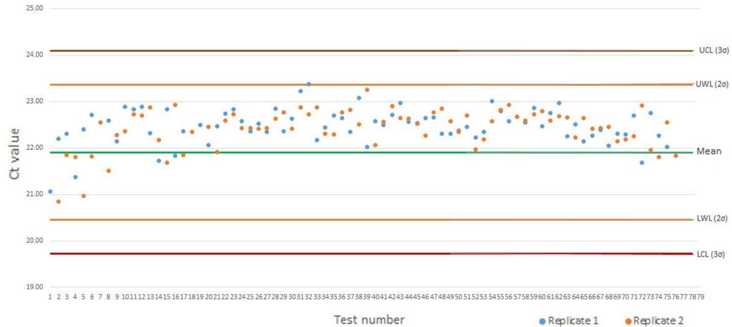
Figure 3-8: Shewhart chart for the biological positive control. The biological positive control was included on every APPV RT-qPCR assay in duplicate. The upper (UWL) and Lower (LWL) warning limits (red lines) show variation of 2 standard deviations from the mean (green line) whereas the Upper (UCL) and lower (LCL) control limits (orange lines) indicate 3 standard deviations variation from the mean.
