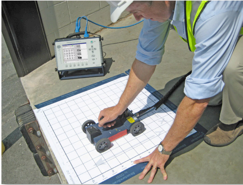
Figure 23: Photograph showing concrete evaluation using a high-frequency GSSI antenna (Geophysical Survey Systems, Inc., 2001)
