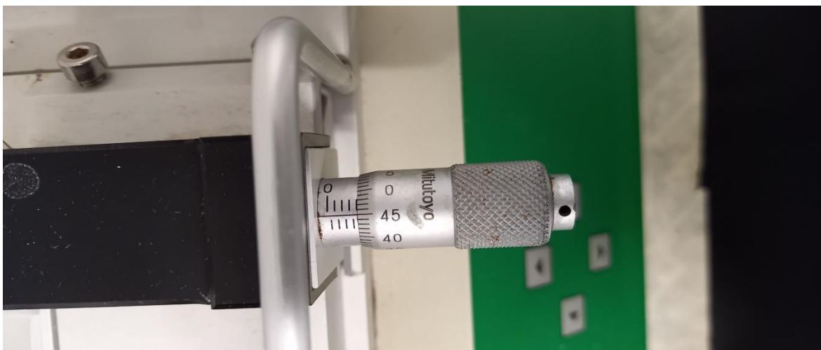
Fig 6. Detail of a micrometre. By turning it anti clockwise it allows to increase the distance between the pins or jaws, stretching the wall of the mounted artery. The sleeve has a total length of 25 mm divided into fifty equal parts, while the thimble is divided into fifty equal parts, a complete turn of the thimble equals 0.5 mm on the sleeve. The reading in the image is 3.5 mm on the sleeve to which are added 0.45 mm from the thimble, equalling 3.95 mm (3950 \mu\text{m} ).
