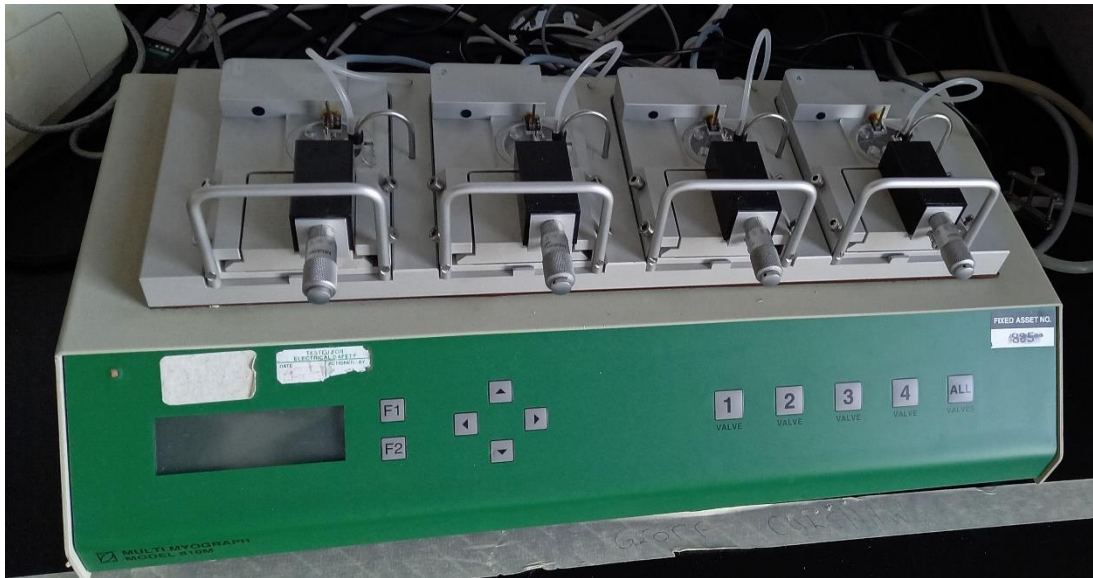
Fig 4. Multiwire Myograph System 610 M (DMT) at The Roslin Institute, with four wells which can be equipped with pin or jaws.
