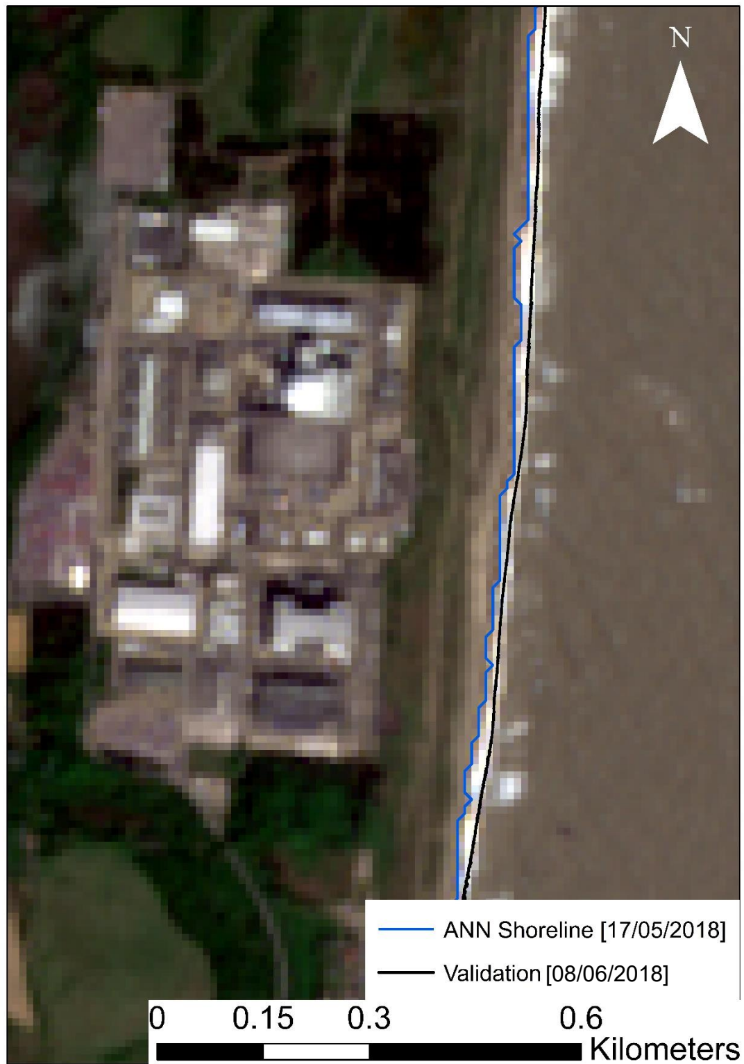
Figure 42: Comparison of ANN-derived shoreline (blue line) and validation shoreline (black line) at Sizewell on 17/05/2018. The validation shoreline, obtained from drone-based shorelines on 08/06/2018, is tidally corrected to align with the date of the captured shoreline.
