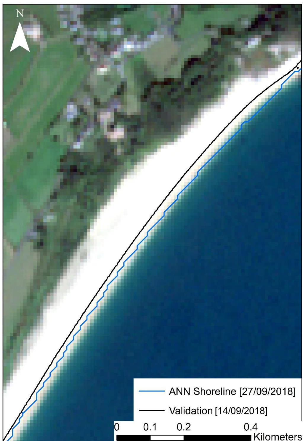
Figure 33: Comparison of ANN-derived shoreline (blue line) and validation shoreline (black line) at Slapton Sands on 27/09/2018. The validation shoreline, obtained from LiDAR data on 12/09/2018, is tidally corrected to align with the date of the captured shoreline.
