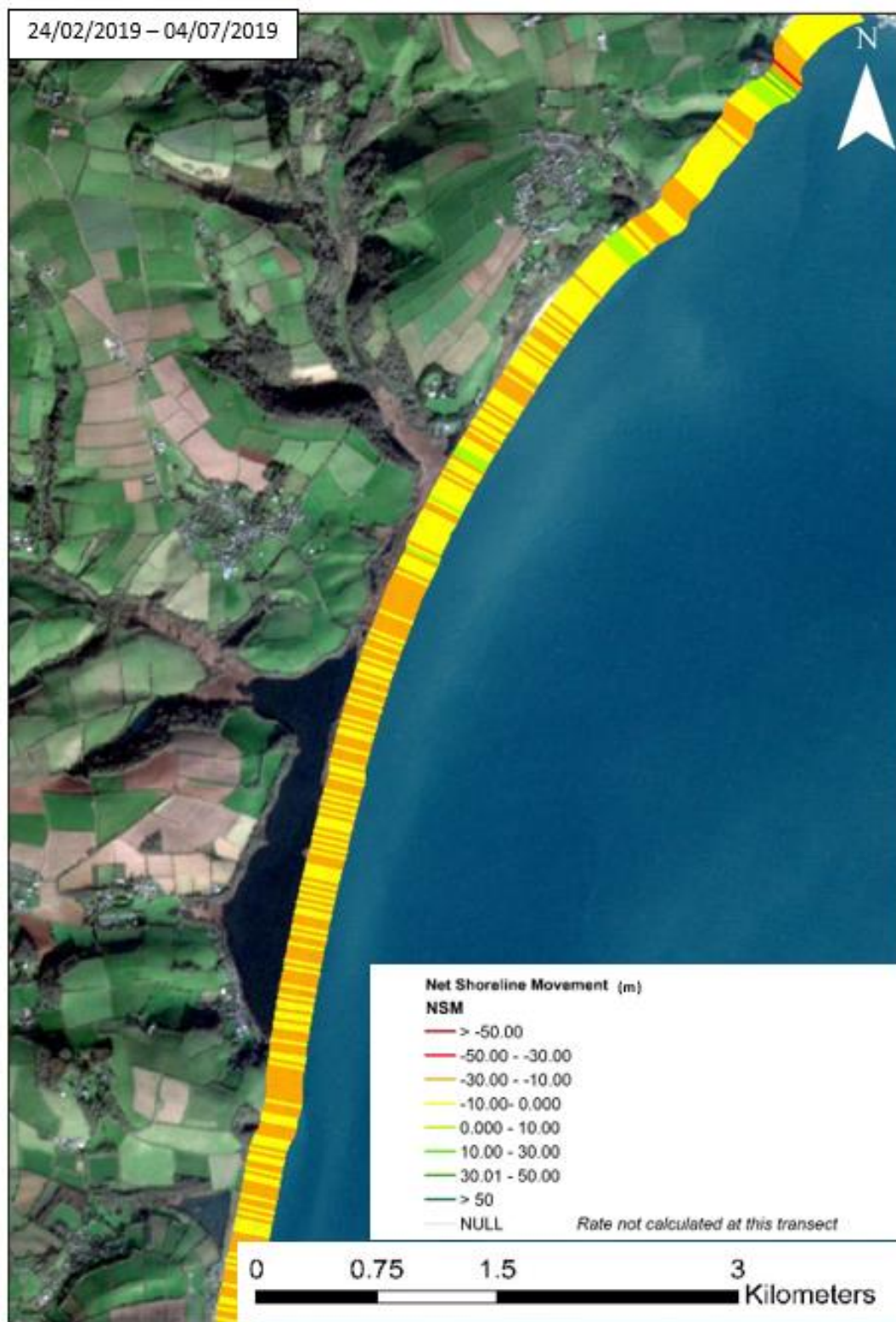
Figure 57: NSM at Start Bay (50°17'0.76"N, 3°38'46.44"W) between 24/02/2019 - 04/09/2019.
