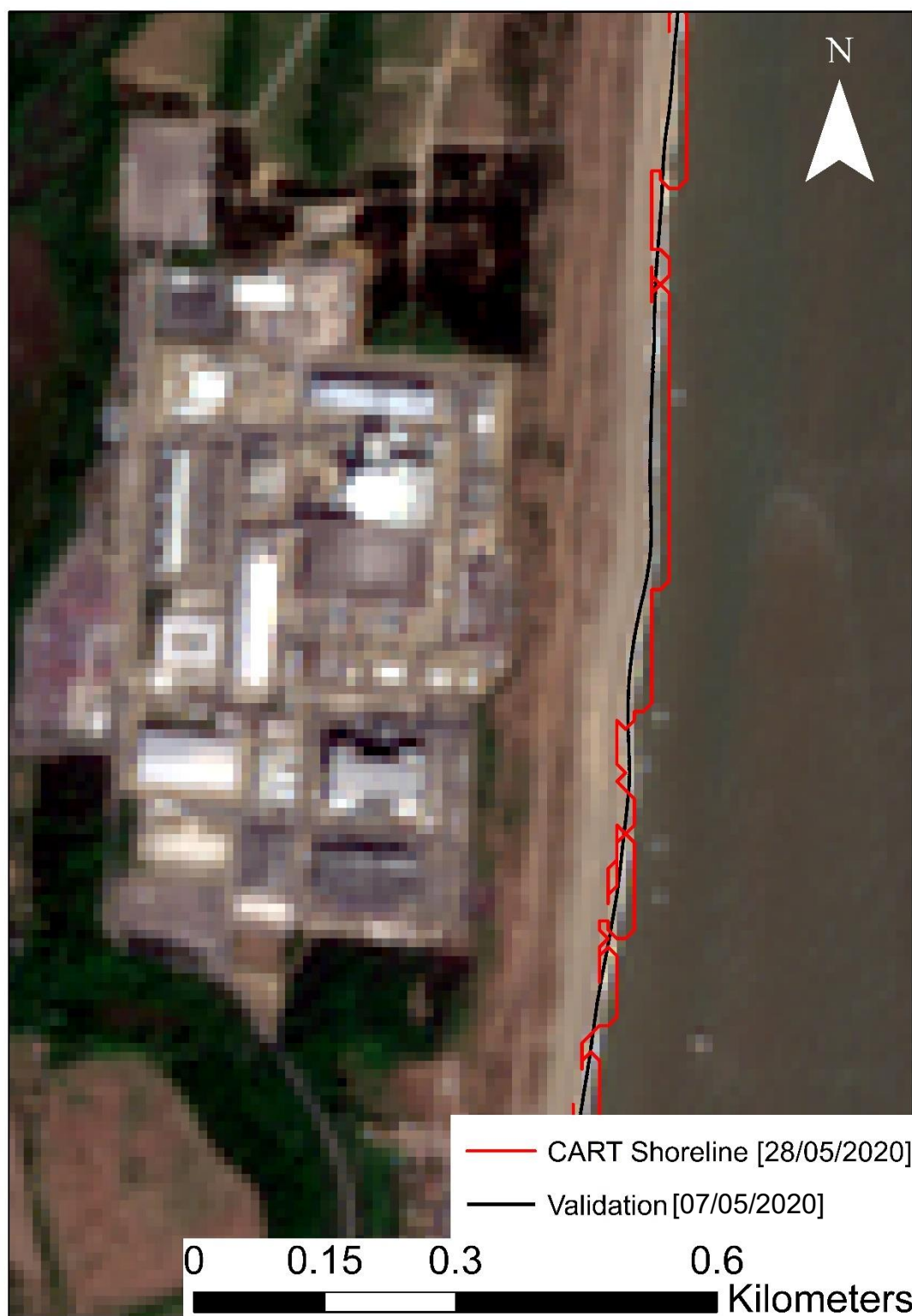
Figure 29: Comparison of CART-derived shoreline (red line) and validation shoreline (black line) at Sizewell on 28/05/2020. The validation shoreline, obtained from drone-based shorelines from 07/05/2020, is tidally corrected to align with the date of the captured shoreline.
