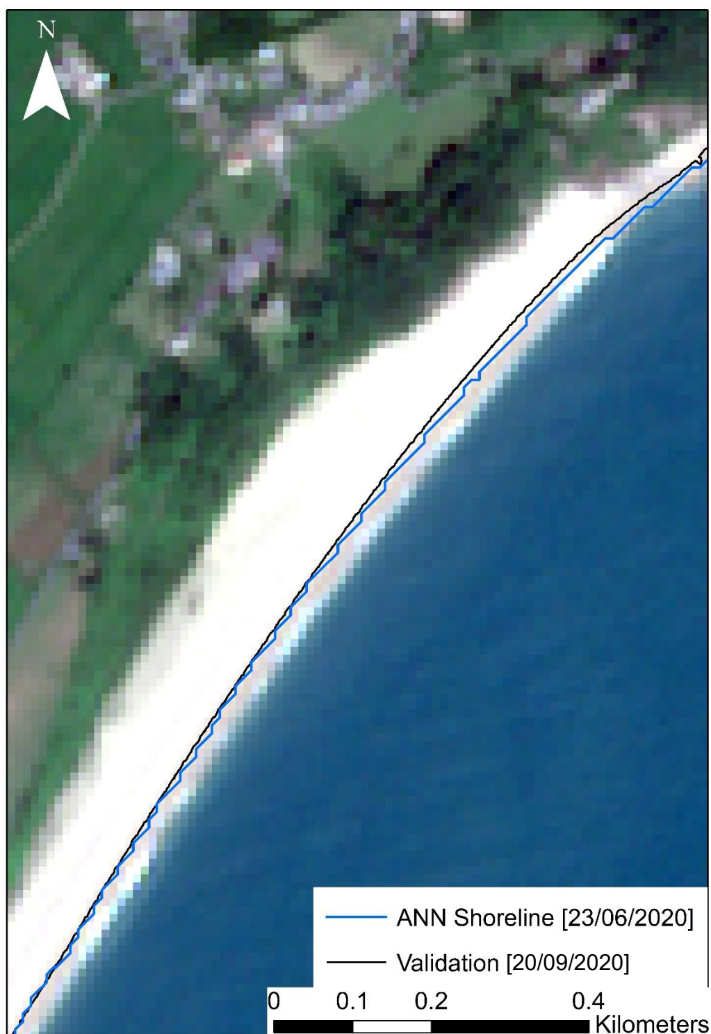
Figure 35: Comparison of ANN-derived shoreline (blue line) and validation shoreline (black line) at Slapton Sands on 23/06/2020. The validation shoreline, obtained from LiDAR data on 20/09/2020, is tidally corrected to align with the date of the captured shoreline.
