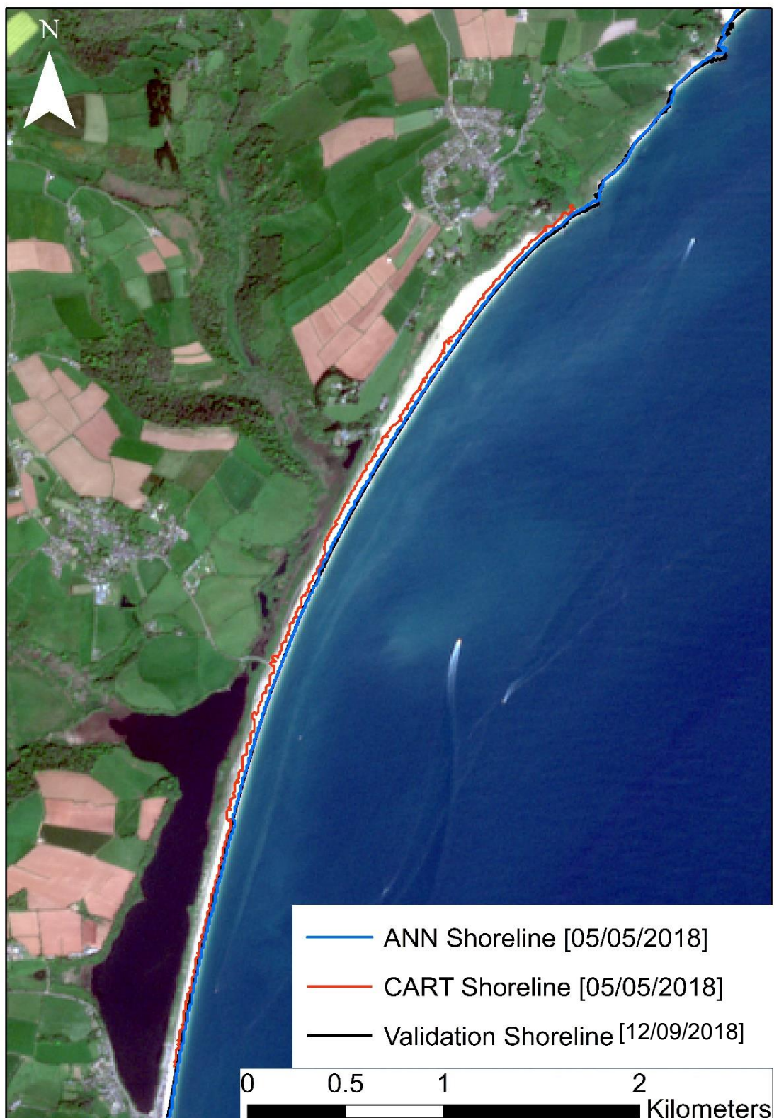
Figure 47: Comparison between the extracted CART shoreline (red), the ANN shoreline (blue) and the validation shoreline (black) observed at Start Bay on 12/09/2018.
