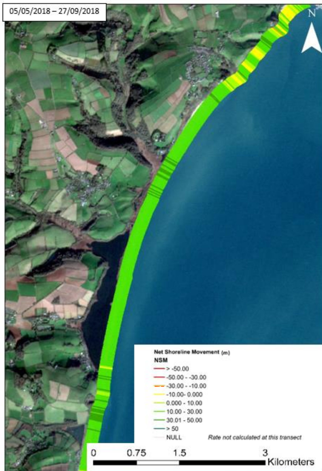
Figure 55: NSM at Start Bay (50°17'0.76"N, 3°38'46.44"W) between 05/05/2018 and 27/09/2018.
