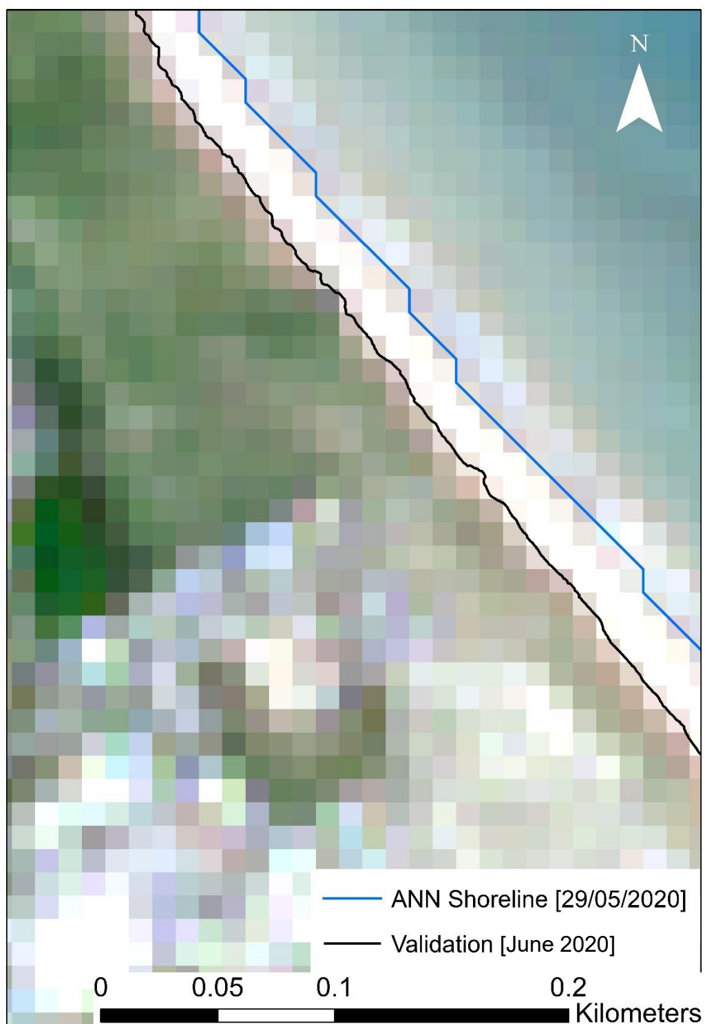
Figure 40: Comparison of ANN-derived shoreline (blue line) and validation shoreline (black line) at Aldbrough on 29/05/2020. The validation shoreline, obtained from LiDAR data on Jun-2020, is tidally corrected to align with the date of the captured shoreline.
