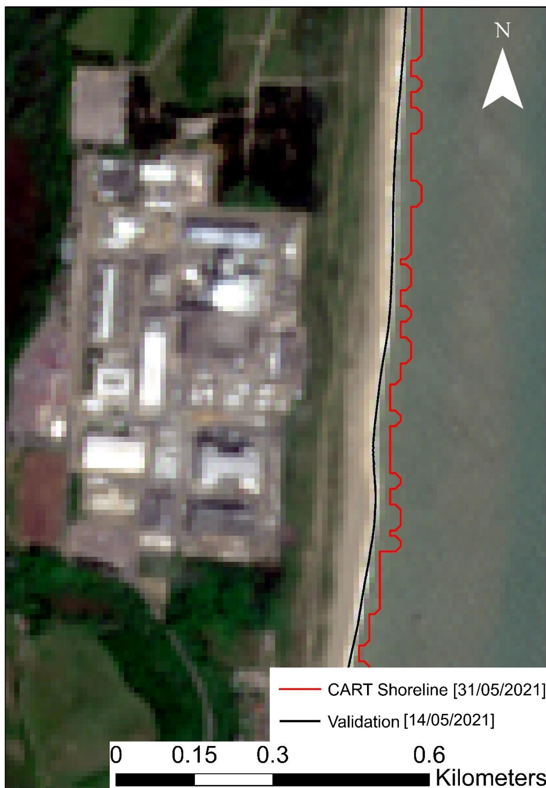
Figure 30: Comparison of CART-derived shoreline (red line) and validation shoreline (black line) at Sizewell on 31/05/2021. The validation shoreline, obtained from drone-based shorelines from 14/05/2021, is tidally corrected to align with the date of the captured shoreline
