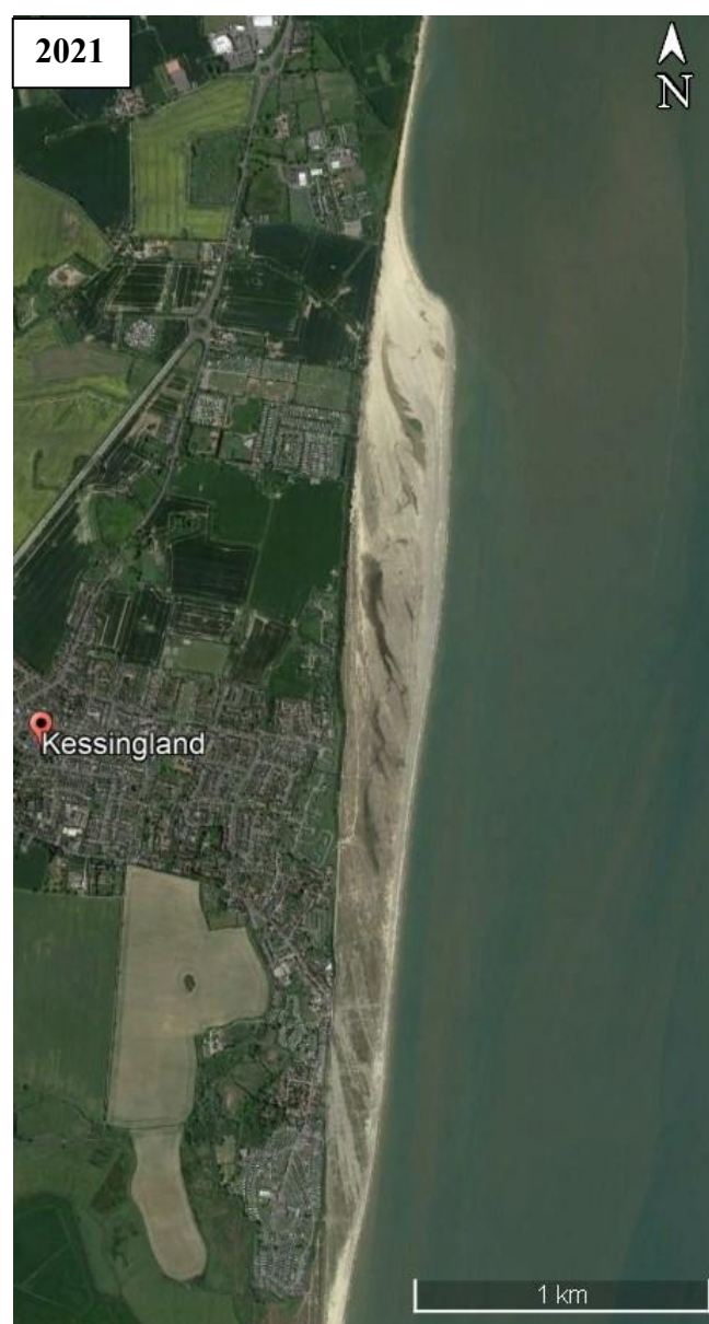
Figure 79: Evolution of Kessingland Ness between 1945 and 2021. The growth of the Ness is seen moving north, with the sediment input coming from the south from Benacre. Over the period shown, the beach has extended 3km northwards (Source: Google Earth).
