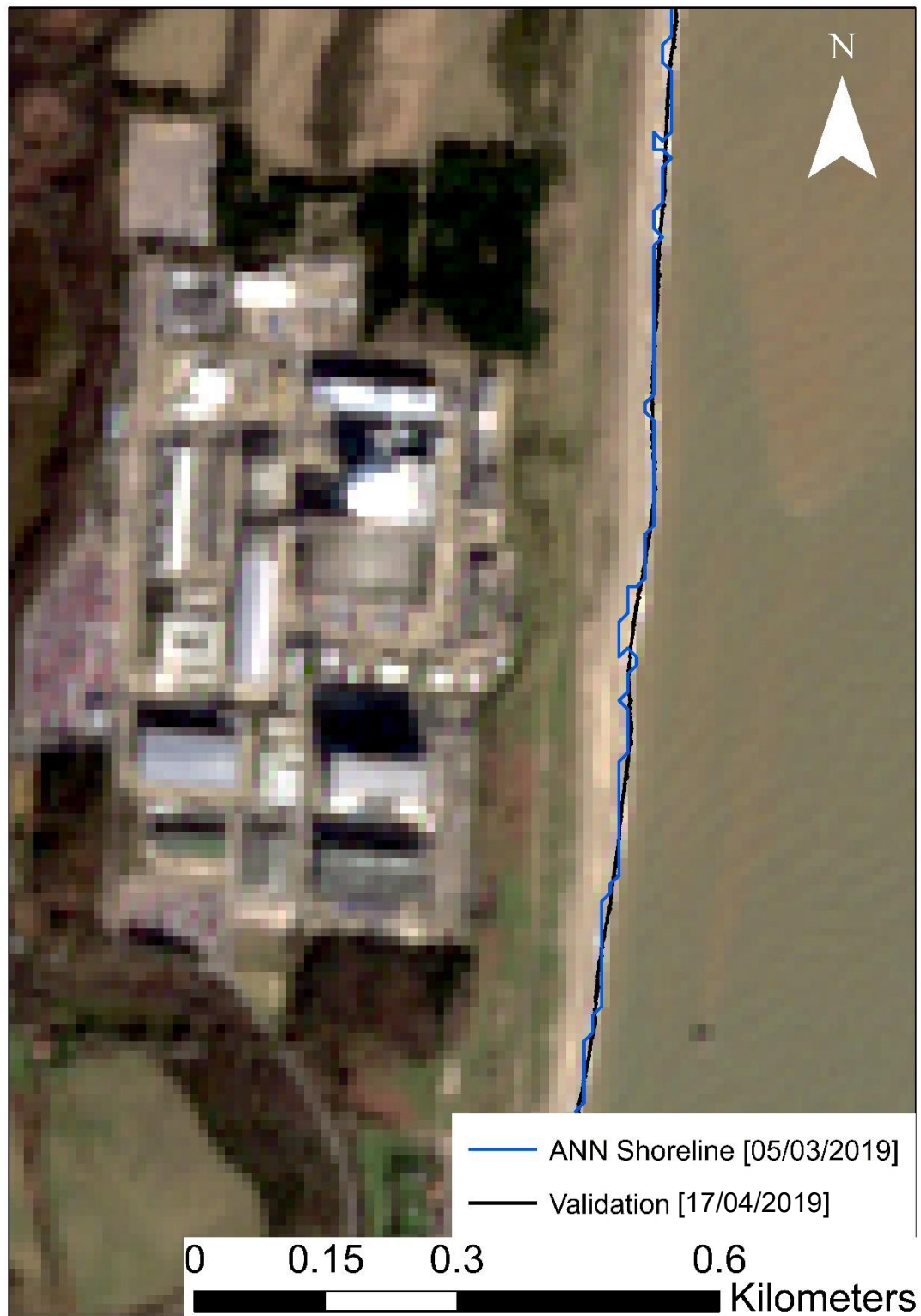
Figure 43: Comparison of ANN-derived shoreline (blue line) and validation shoreline (black line) at Sizewell on 05/03/2019. The validation shoreline, obtained drone-based shorelines on 17/04/2019, is tidally corrected to align with the date of the captured shoreline.
