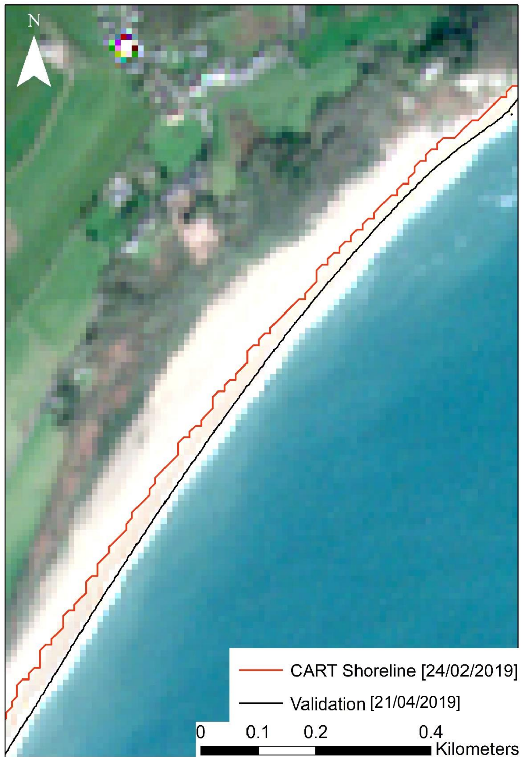
Figure 19: Comparison of CART-derived shoreline (red line) and validation shoreline (black line) at Slapton Sands on 24/02/2019. The validation shoreline, obtained from LiDAR data on 21/04/2019, is tidally corrected to align with the date of the captured satellite image.
