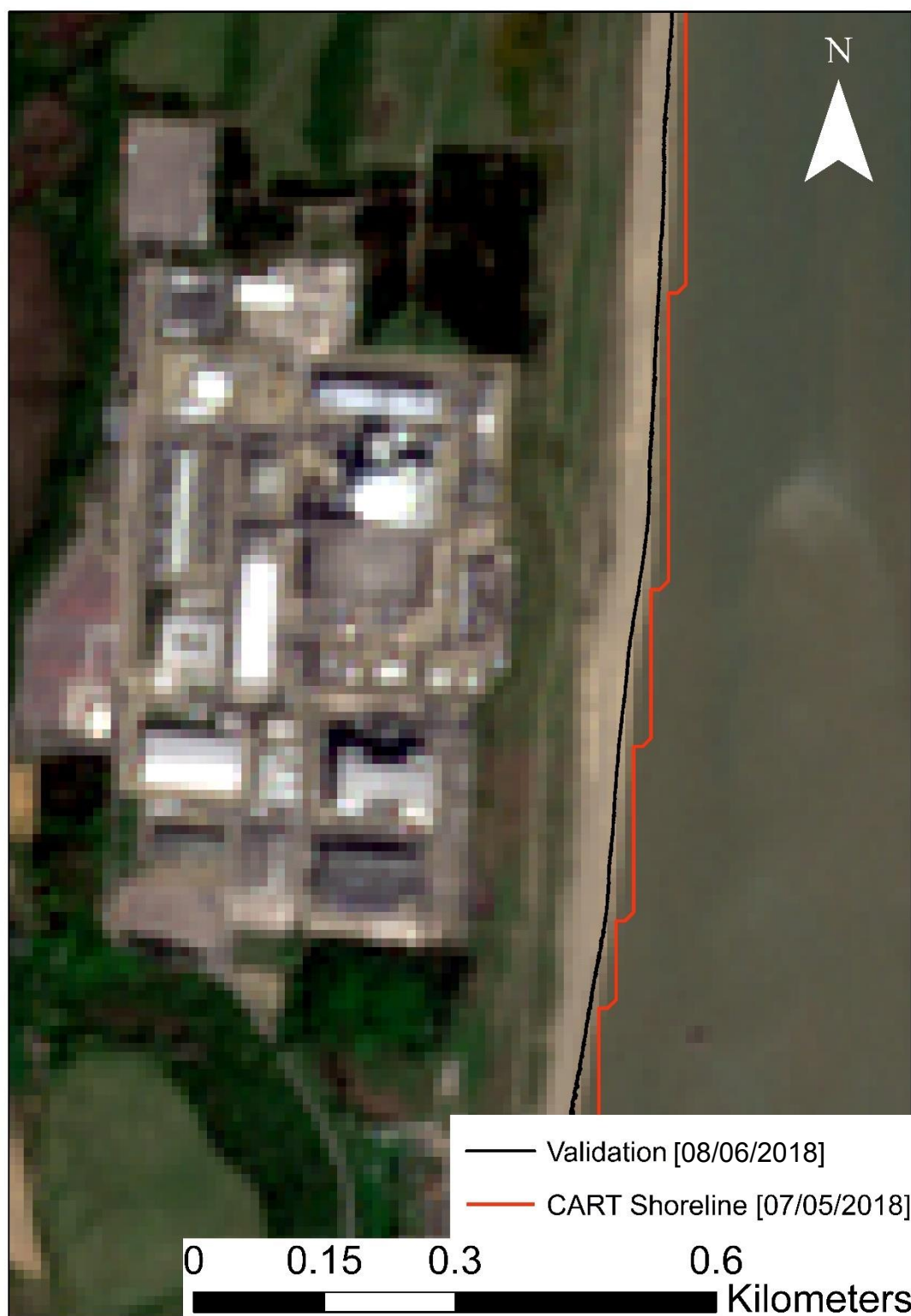
Figure 27: Comparison of CART-derived shoreline (red line) and validation shoreline (black line) at Sizewell on 07/05/2018. The validation shoreline, obtained from drone-based shorelines from 08/06/2018, is tidally corrected to align with the date of the captured shoreline.
