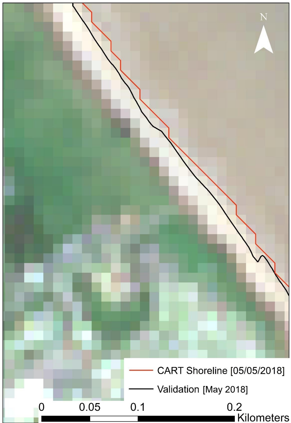
Figure 22: Comparison of CART-derived shoreline (red line) and validation shoreline (black line) at Aldbrough on 05/05/2018. The validation shoreline, obtained from LiDAR data from May 2018, is tidally corrected to align with the date of the captured shoreline.
