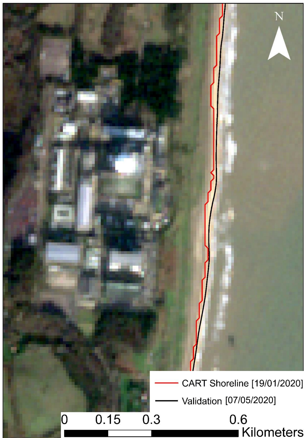
Figure 28: Comparison of CART-derived shoreline (red line) and validation shoreline (black line) at Sizewell on 19/01/2020. The validation shoreline, obtained from drone-based shorelines from 07/05/2020, is tidally corrected to align with the date of the captured shoreline.
