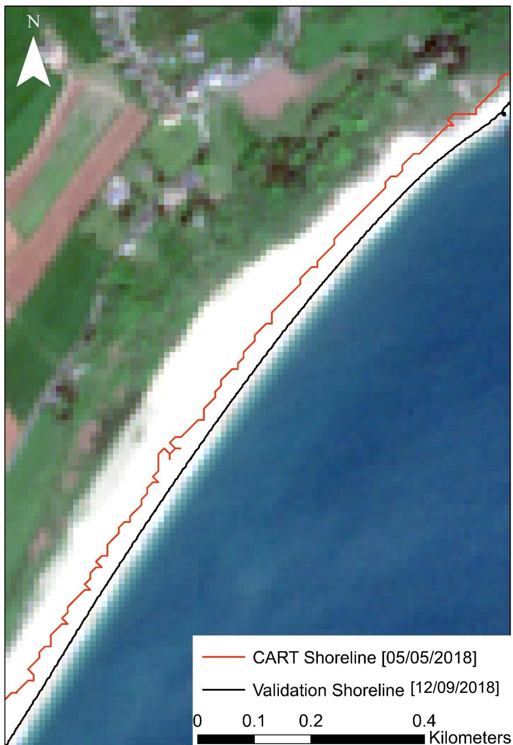
Figure 17: Comparison of CART-derived shoreline (red line) and validation shoreline (black line) at Slapton Sands on 05/05/2018. The validation shoreline, obtained from LiDAR data on 12/09/2018, is tidally corrected to align with the date of the captured satellite image.
