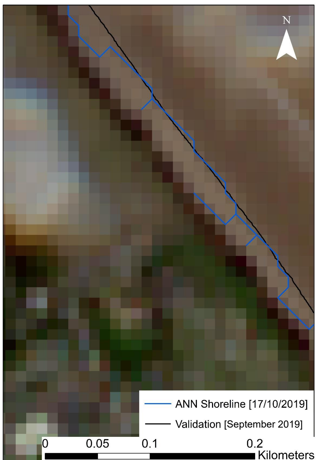
Figure 39: Comparison of ANN-derived shoreline (blue line) and validation shoreline (black line) at Aldbrough on 17/10/2019. The validation shoreline, obtained from LiDAR data on Sept-2019, is tidally corrected to align with the date of the captured shoreline.
