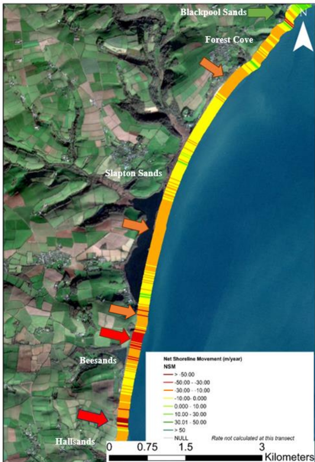
Figure 53: NSM at Start Bay ( 50^{\circ}17'0.76''\text{N} , 3^{\circ}38'46.44''\text{W} ) between 2016 - 2021. Arrows indicate the areas of erosion (red and orange) and accretion (green) based on the rate of change during the study period. The red arrows highlight significant NSM of the shorelines in Hallsands and Beesands. The orange arrows highlight the NSM of the shorelines in Slapton Sands and the green arrow indicates the area with net accretion in Blackpool Sands.
