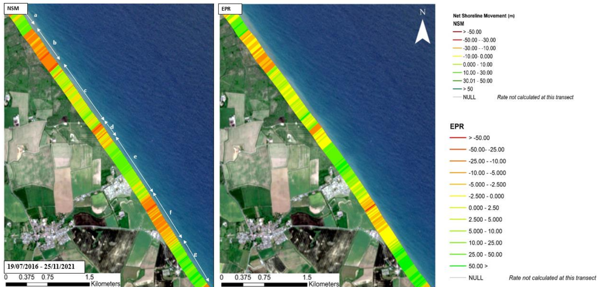
Figure 64: NSM and EPR along the Hull coastline near Aldbrough between 2016 and 2020. Sections a-g highlight the seaward and landward pattern of change over the time period.
