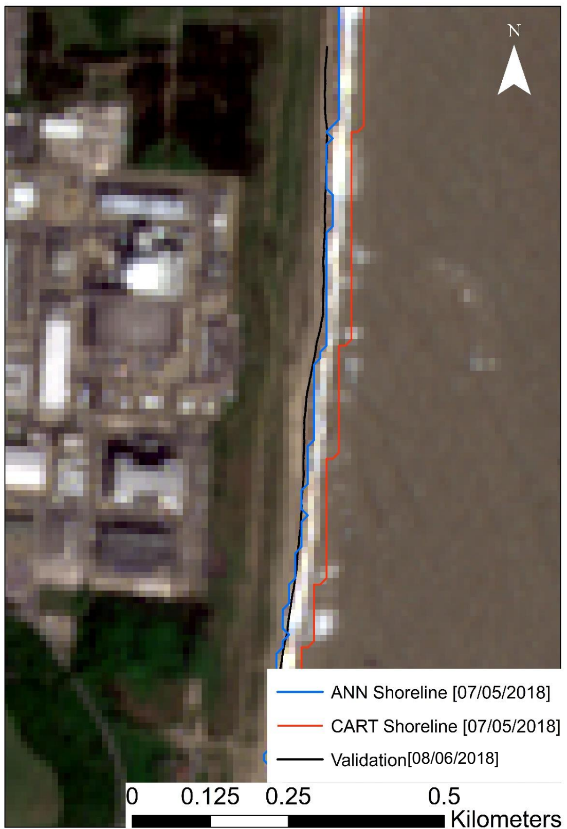
Figure 49: Comparison between the extracted CART shoreline (red), the ANN shoreline (blue) and the validation shoreline (black) observed at Sizewell on 08/06/2018.
