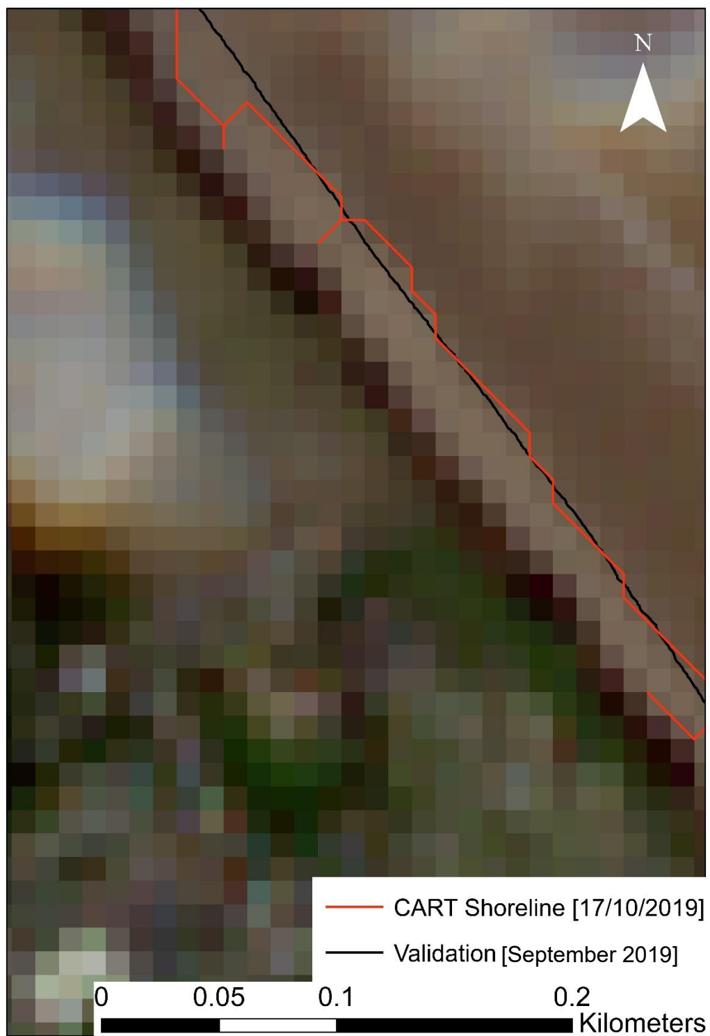
Figure 24: Comparison of CART-derived shoreline (red line) and validation shoreline (black line) at Aldbrough on 17/10/2019. The validation shoreline, obtained from LiDAR data from Sept-2019, is tidally corrected to align with the date of the captured shoreline.
