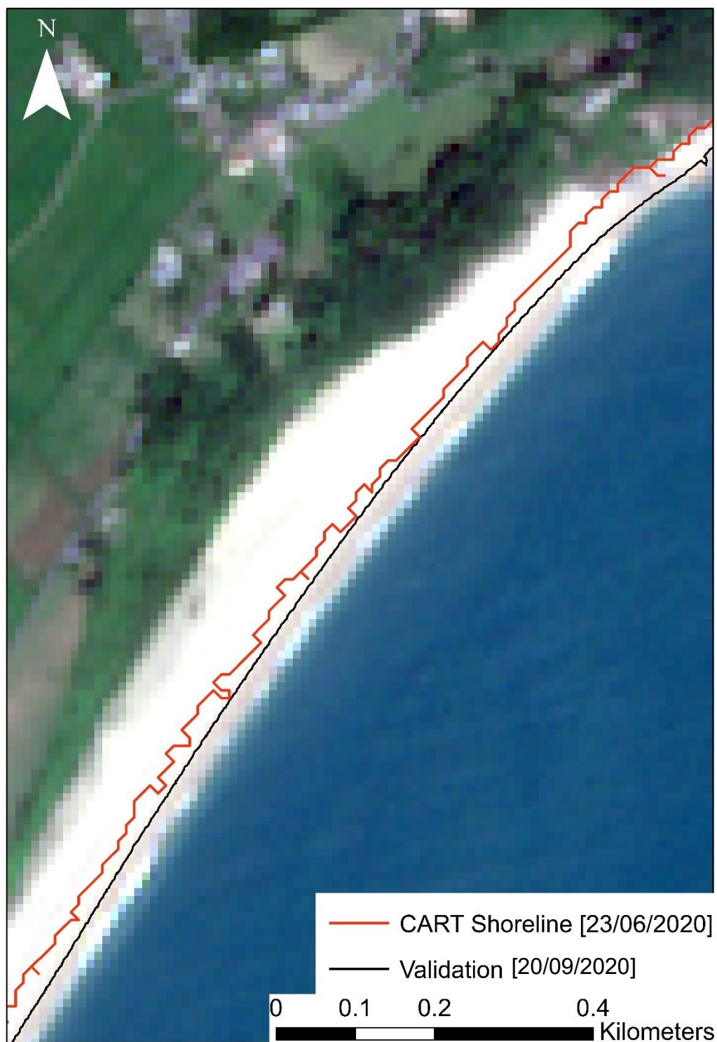
Figure 20: Comparison of CART-derived shoreline (red line) and validation shoreline (black line) at Slapton Sands on 23/06/2020. The validation shoreline, obtained from LiDAR data on 20/09/2020, is tidally corrected to align with the date of the captured shoreline.
