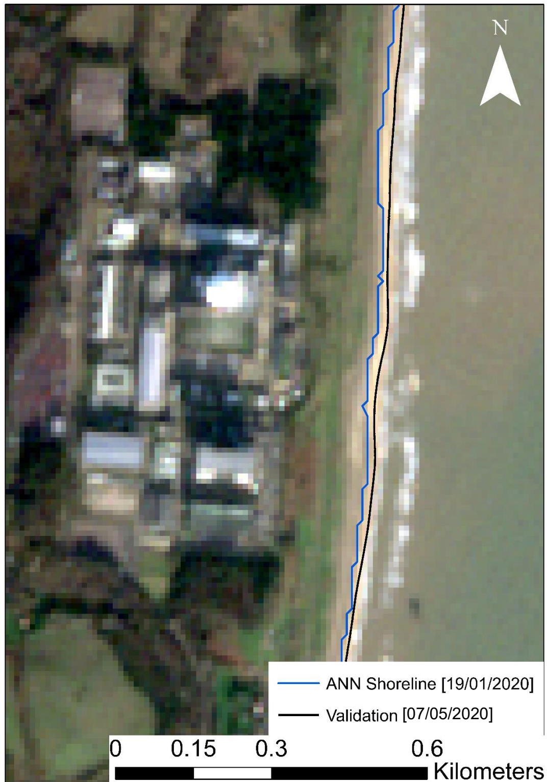
Figure 44: Comparison of ANN-derived shoreline (blue line) and validation shoreline (black line) at Sizewell on 19/01/2020. The validation shoreline, obtained from drone-based shorelines on 07/05/2020, is tidally corrected to align with the date of the captured shoreline.
