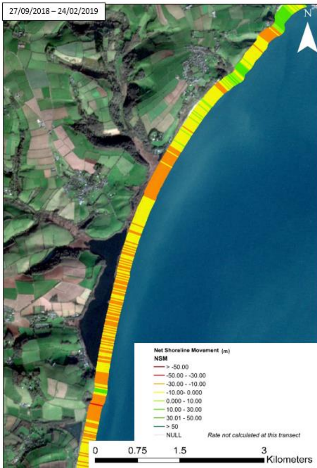
Figure 56: NSM at Start Bay (50°17'0.76"N, 3°38'46.44"W) between 27/09/2018 and 24/02/2019.
