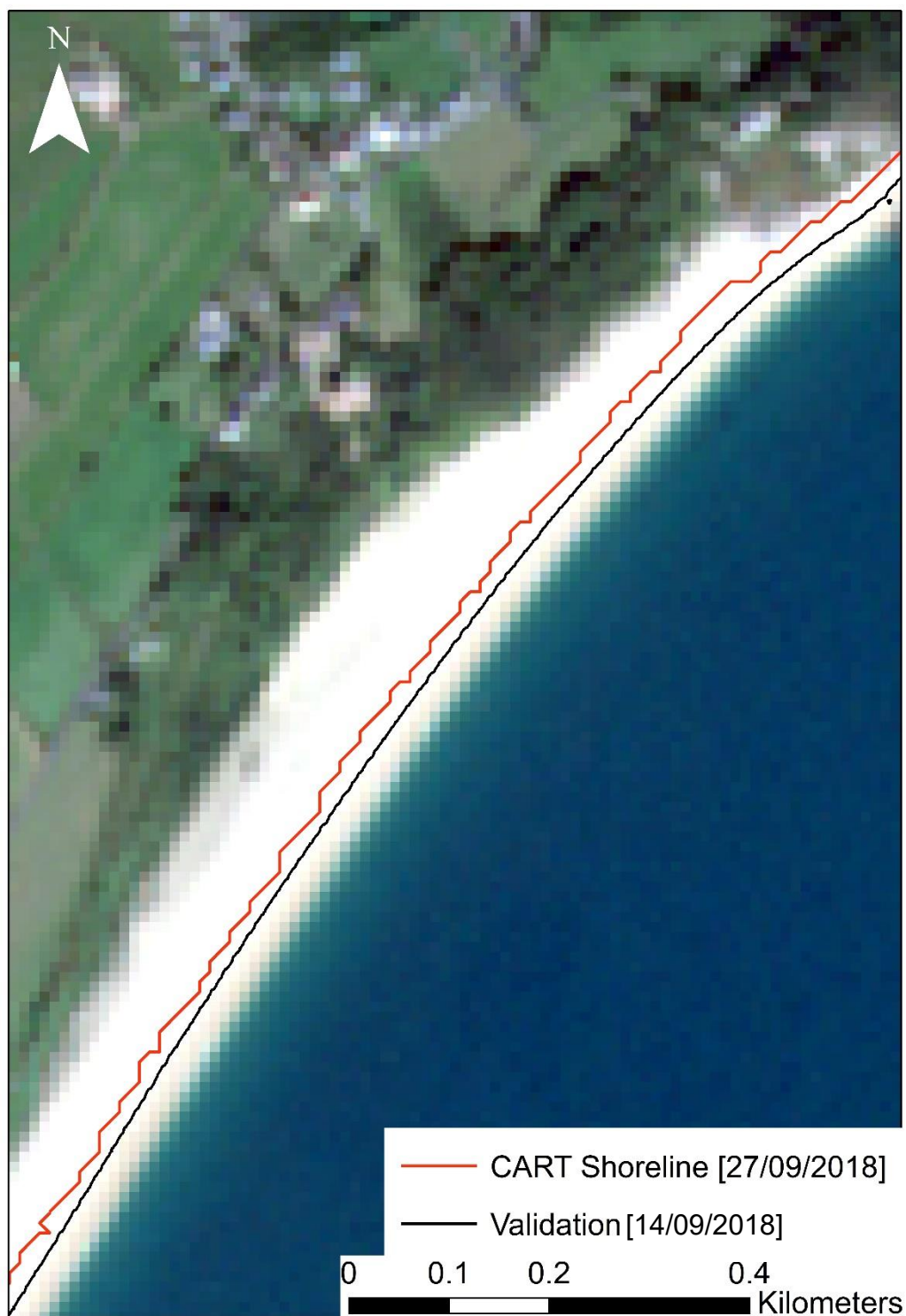
Figure 18: Comparison of CART-derived shoreline (red line) and validation shoreline (black line) at Slapton Sands on 27/09/2018. The validation shoreline, obtained from LiDAR data on 14/09/2018, is tidally corrected to align with the date of the captured satellite image.
