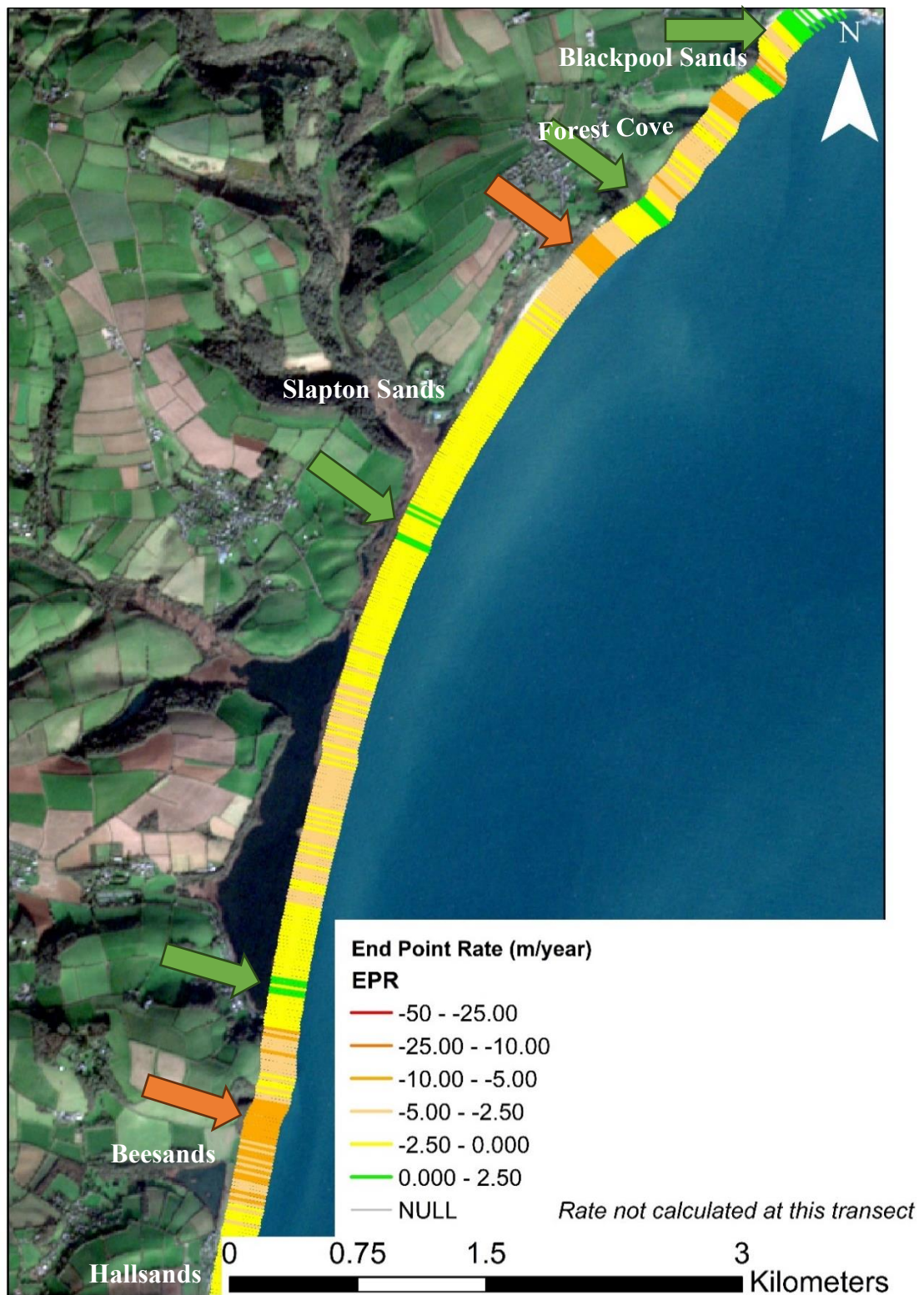
Figure 54: EPR at Start Bay (50°17'0.76"N, 3°38'46.44"W) between 2016-2021. Arrows indicate the areas of erosion (red and orange) and accretion (green) based on the rate of change during the study period. The orange arrows highlight the negative EPR in Beesands and Slapton Sands. The green arrows show significant positive EPR in areas of Slapton Sands and Blackpool Sands.
