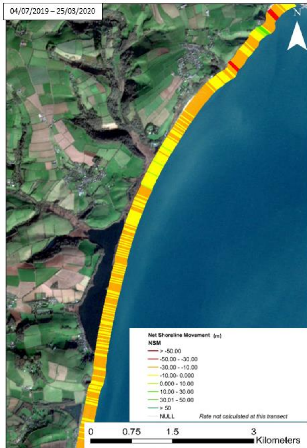
Figure 58: NSM at Start Bay (50°17'0.76"N, 3°38'46.44"W) between 04/07/2019 and 25/03/2020.
