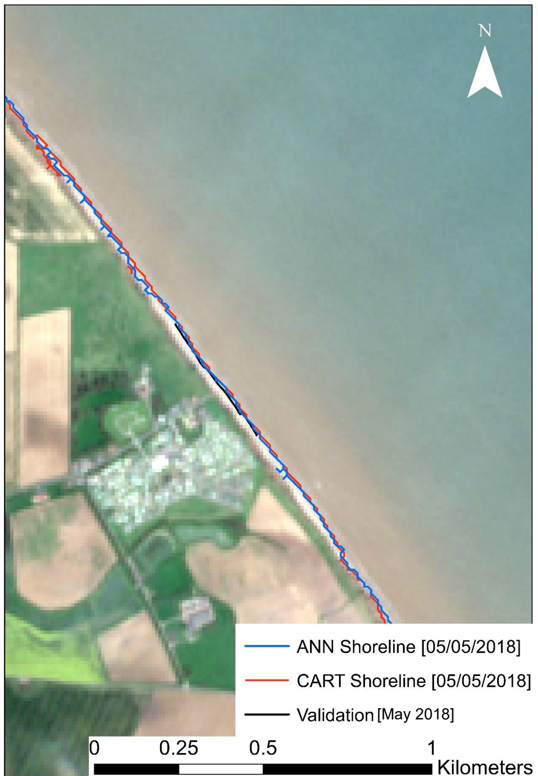
Figure 48: Comparison between the extracted CART shoreline (red), the ANN shoreline (blue) and the validation shoreline (black) observed at Aldbrough in May 2018.
