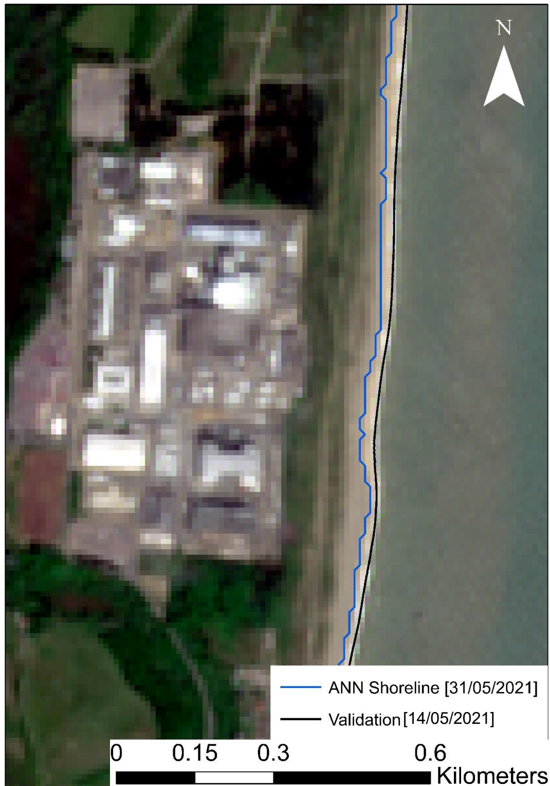
Figure 45: Comparison of ANN-derived shoreline (blue line) and validation shoreline (black line) at Sizewell on 31/05/2021. The validation shoreline, obtained from drone-based shorelines on 14/05/2021, is tidally corrected to align with the date of the captured shoreline.
