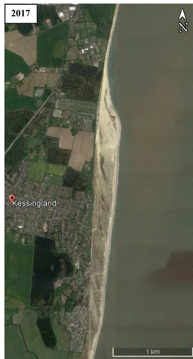
Figure 79: Evolution of Kessingland Ness between 1945 and 2021. The growth of the Ness is seen moving north, with the sediment input coming from the south from Benacre. Over the period shown, the beach has extended 3km northwards (Source: Google Earth).
