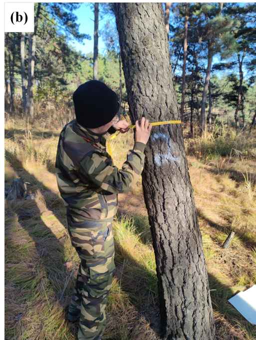
Figure 1.5: Measurement of DBH at a forest plot using a diameter tape. (a) Diameter tape, (b) Measurement of DBH at a field plot.
