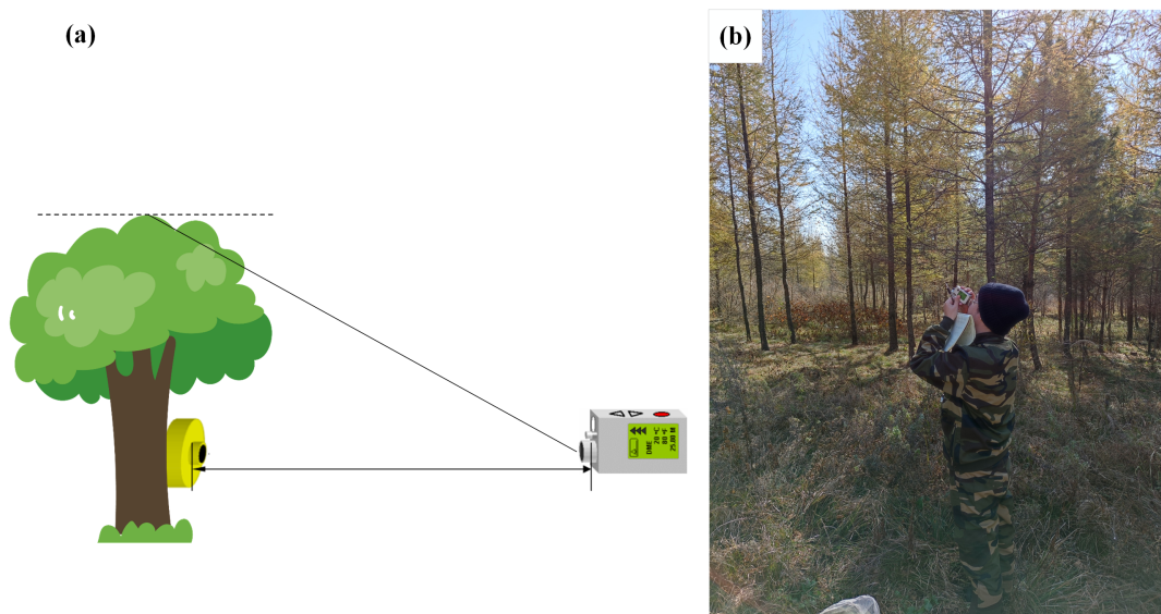
Figure 1.6: Measurement of tree height using laser rangefinders and transponder. (a) Laser rangefinder and transponder, (b) Measurement of tree height at a field plot.
