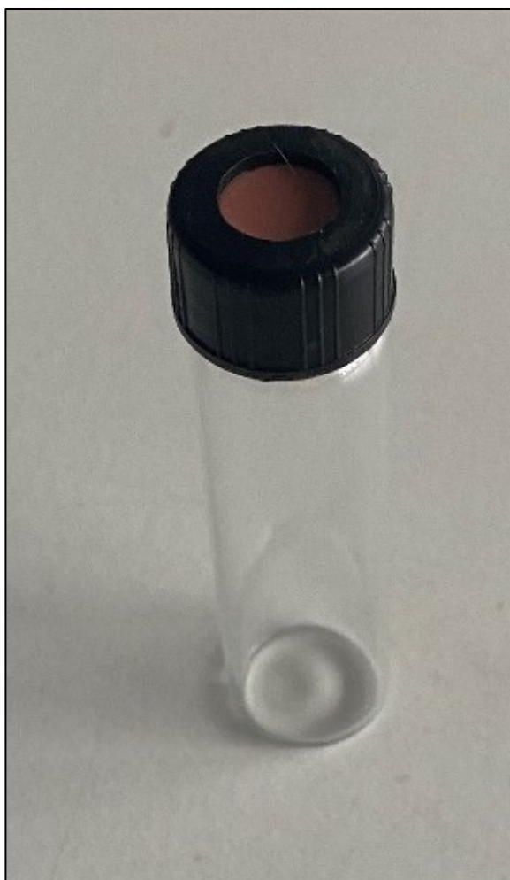
Figure 3.5 – Pressure-resistant Teflon-capped reaction vial used in fatty acid extraction method
