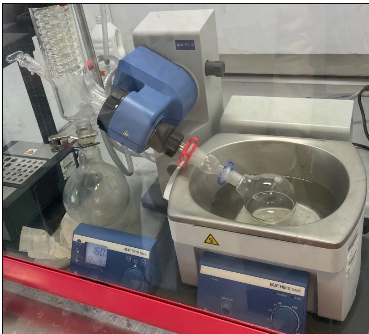
Figure 3.6 – 250 ml round-bottomed flask attached to rotary evaporator using manufacturer adaptors
