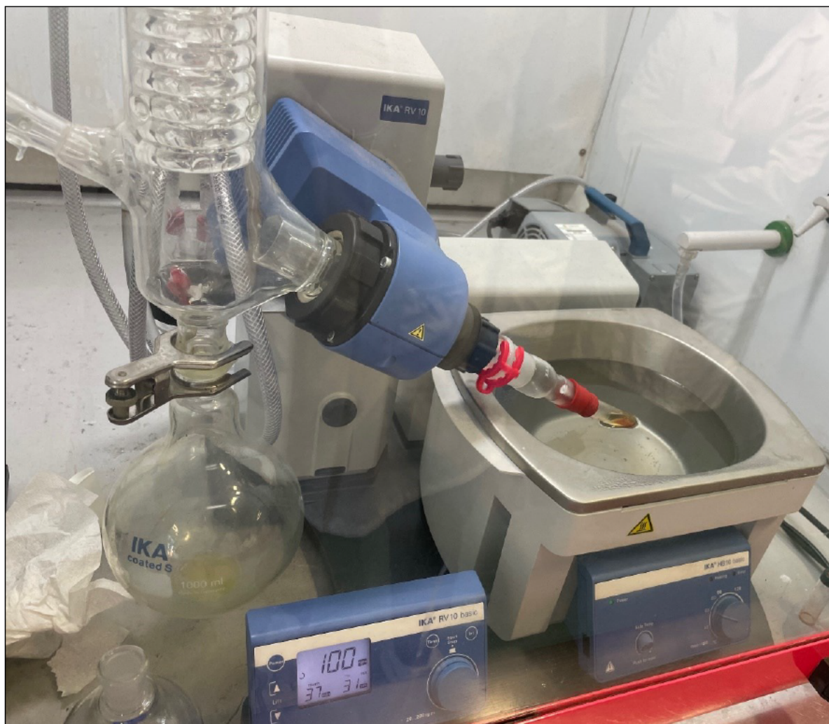
Figure 3.7 - Modified adapter to fit small reaction vials to the rotary evaporator
