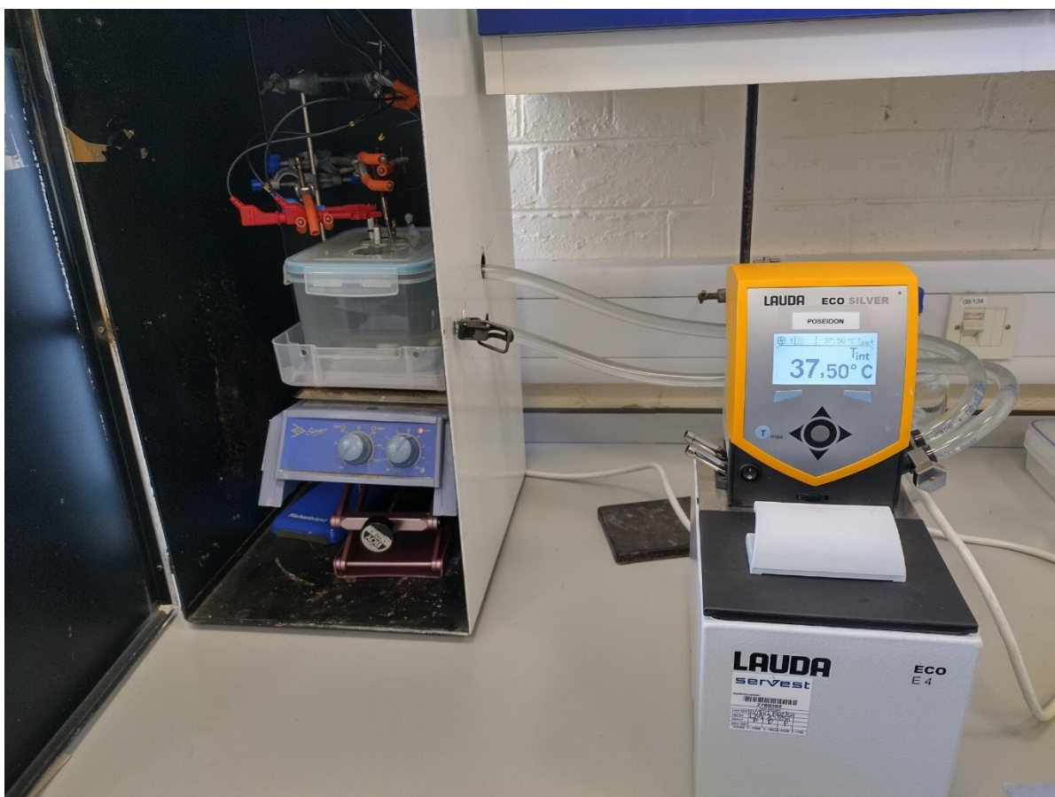
Figure 2.18 External view of general experimental setup for electrochemistry in this work. Temperature control within the in-house extended water bath (left) is provided by a coupled commercial water bath outside the Faraday cage (right).
