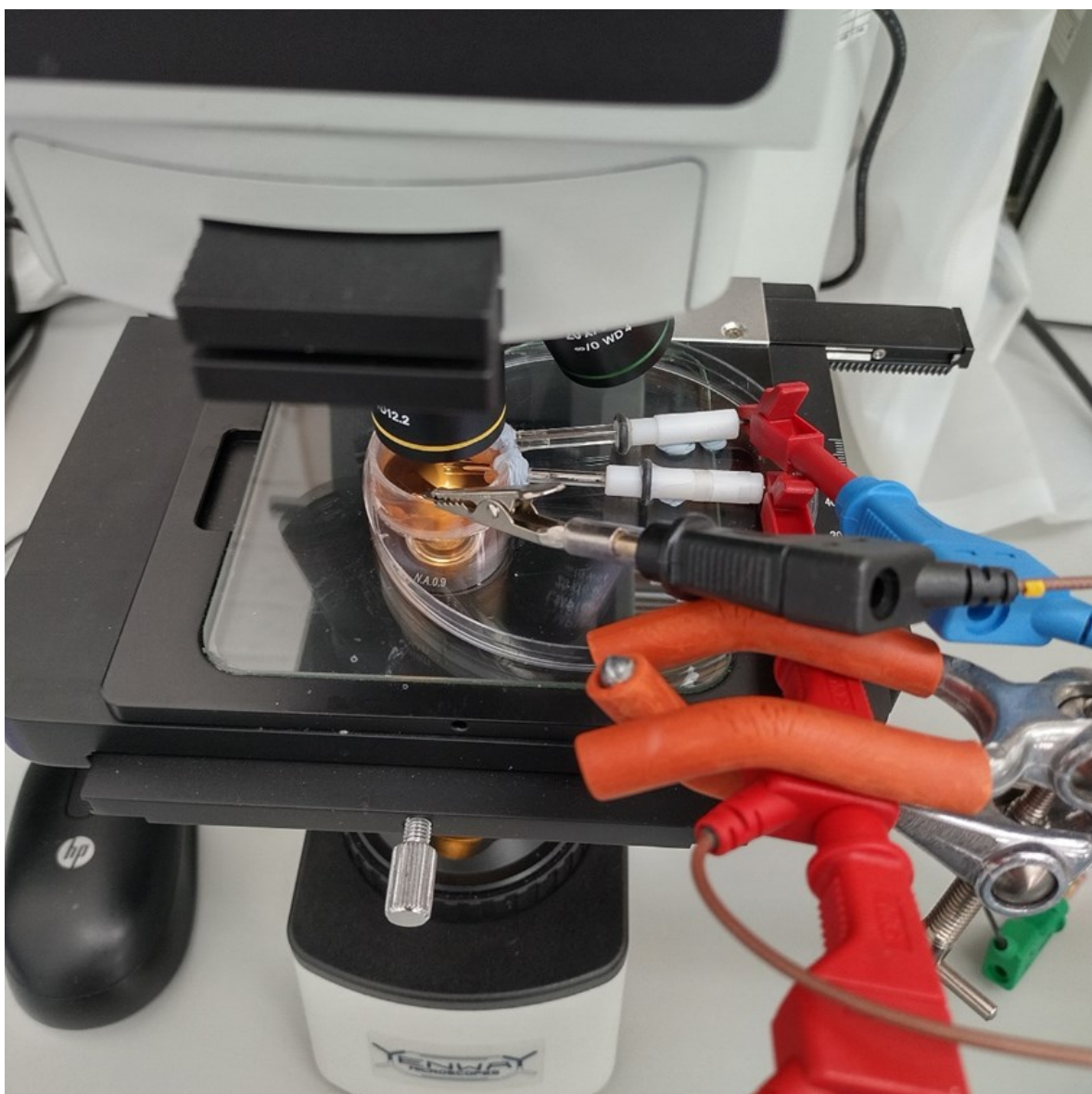
Figure 2.22 Experimental setup for 3 hour potentiostatic Carb-Ala gel growth experiments. Features petri dish with open-topped ~5 mL vessel, sealed with epoxy resin to base of dish. The three-electrode system features a Pt disc microelectrode (25 \mu\text{m} ) and Ag/AgCl/Cl - reference electrode (both fixed in slots at the side of the vessel and sealed with silicone rubber), with a Pt sputter-coated silicon chip counter electrode (rested in the vessel). The vessel is filled with 5 mL 10 mg/mL Carb-Ala gelator solution.
