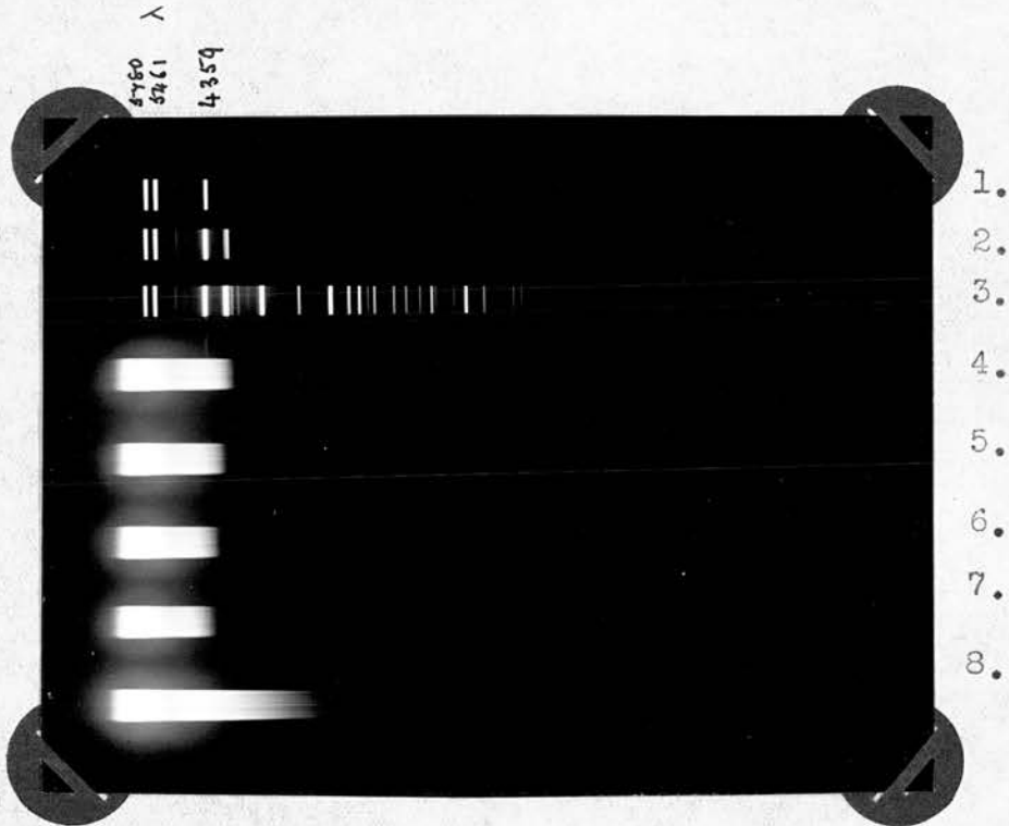
Absorption Spectra of 1 -Menthyl 2:4-Dinitrophenyl Ether, 2 % solution in acetone. (Panchromatic Plate)
