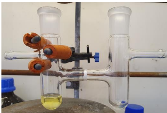
Figure 7.3 – Photograph of H-tube apparatus for selective stripping experiments.
