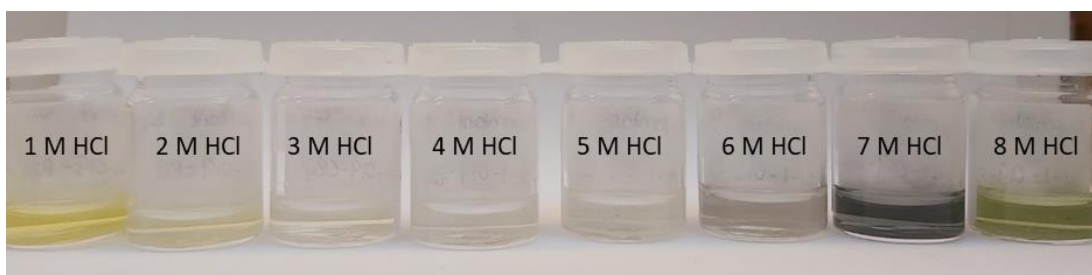
Figure 3.47 – Photograph of the supernatants resulting from L 21 contacted with 0.01 M HAuCl 4 in 1 – 8 M HCl.
