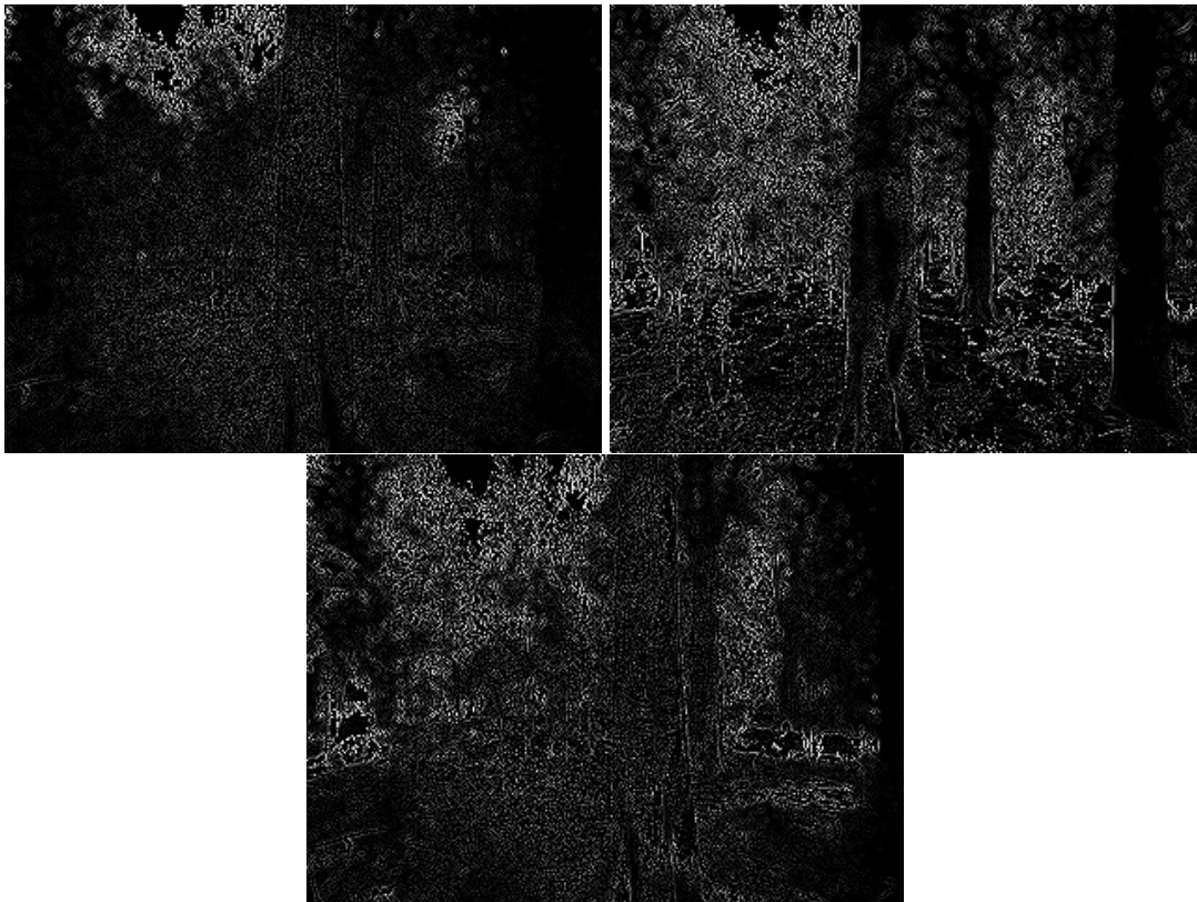
Figure 6.5: Laplacian edge images from the start of simulated sequences under different conditions: Cloud (top left), Winter (top right) and the base condition (bottom). Whiter pixels represent stronger edge values.
