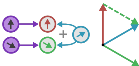
Figure 7.8: Illustrating rules for steering circuits. Rule 1 Compass neuron preferred directions must form a positive basis (Figure 7.7) in order to represent any angle in [0, 360^\circ] . Rule 2 Steering neuron pairs are defined by goal neuron innervation. Coloured boxes indicate paired steering neurons. Rule 3 Steering neuron direction is a weighted sum of the compass neurons sampled. Note that the central steering pair only samples from two compass neurons while the outer pairs sample from three. Equal weighted inputs are used for clarity but this is not required. For larger circuits, this could be more convoluted so long as the remaining rules are obeyed. Rule 4 The sign of the angle between left and right driving steering neurons must be consistent. In the invalid example, the central steering pair will generate turns in the opposite direction to the others. Rule 5 The goal direction represented by a specific goal neuron is the mid-point of the directions of the steering neurons it innervates. Note that this is in turn defined by the combination of compass inputs to a given steering neuron as in rule 3. Rule 6 Resultant goal neuron goal directions must form a positive basis.
