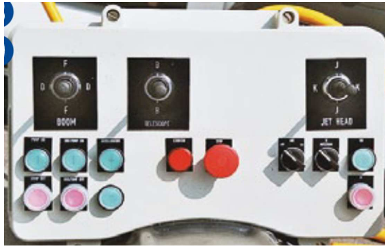
Figure 2.3: The control pad an operator uses to manipulate a MEYCO Oruga Concrete Spraying Unit. Several buttons at the bottom modify operational parameters, and the three joysticks above control the individual joint velocities of the manipulator.
