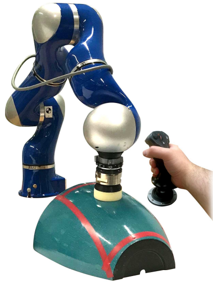
Figure 5.1: Lab mock-up on a KUKA LWR in shared control mode; with online MPC based skill estimation and switching.
