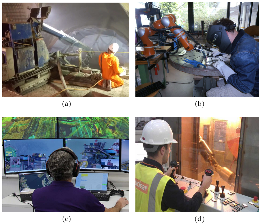
Figure 1.1: Industrial teleoperation tasks such as (a) concrete spraying, (b) welding, (c) remote drone piloting for inspection, and (d) nuclear decommissioning each require highly skilled operators.
