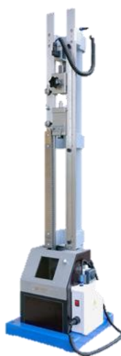
Figure 1.2. BAM fall hammer test
