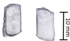
Figure 5.4. Example of a halved post run sample enclosed in 70% silver, 30% palladium capsule. The previously visible green and orange endoliths embedded within the sample are no longer visible.
