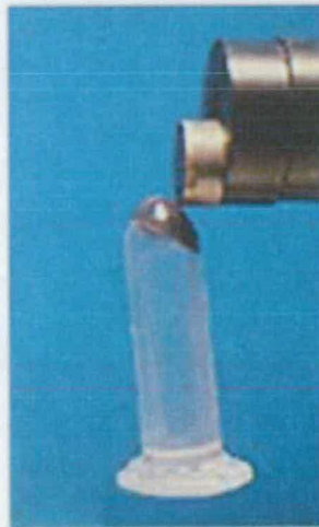
Figure 1.11 A pellet of isolated magnetosomes in a microfuge tube sticking to a permanent magnet. (Plate courtesy of Dirk Schüler).
