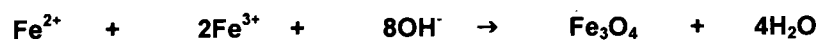
Figure 1.10 A chemical equation representing ion transfer during the co-precipitation of Fe (II) and Fe (III) in alkaline solution.
