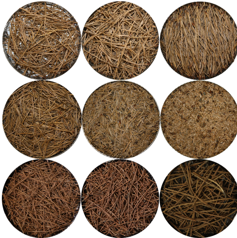
Figure 39: Photos of some of the fuel beds tested. Left to right and top to bottom - Rigida 7.5 g, 15 g, 25 g, 35 g, 60 g, 95 g; Halepensis 15 g; Pinea 15 g; Pinaster 15 g.
