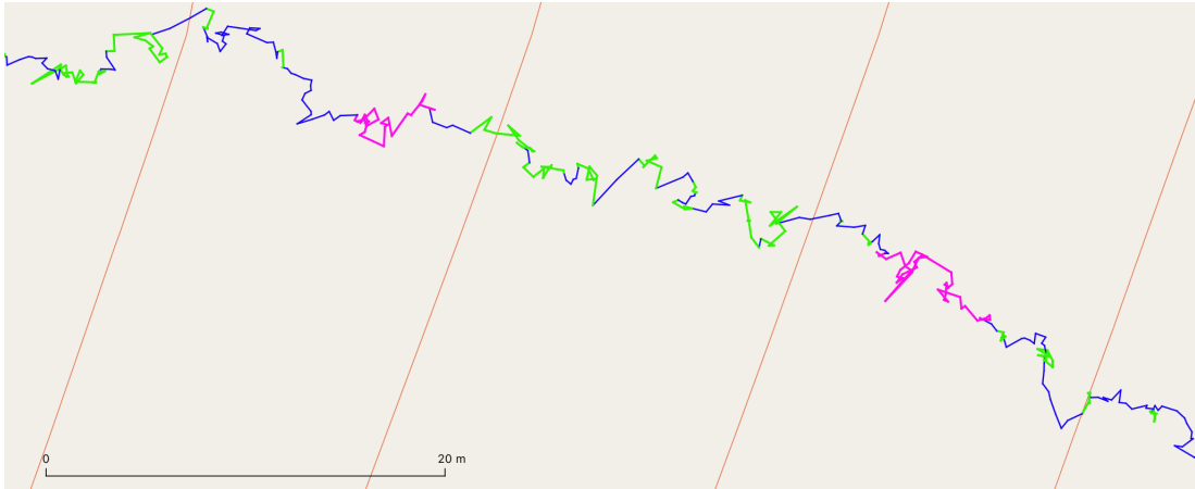
Figure 5.4: A steep section of one of the GPS traces from the fieldwork, with breaks highlighted. Breaks under 30 seconds are coloured green, and breaks over 30 seconds are coloured pink. 10 m contour lines are also shown to indicate hill slope. Background map from OpenStreetMap, visualised using QGIS (see 2.2.5).
