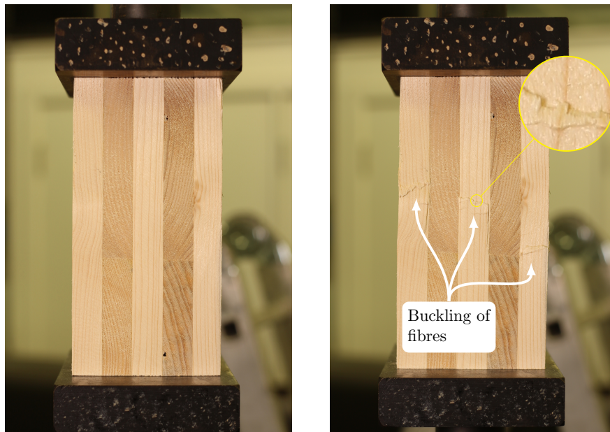
Figure 4.5. Failure mode of a 5-ply polyurethane specimen, as a representative failure mode, in comparison to intact sample before loading commences.
