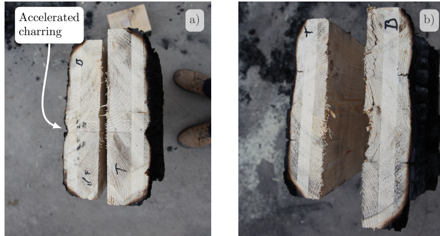
Figure 6.18. Charred profile at mid height cross-section for a) a three ply and b) a five ply sample.
