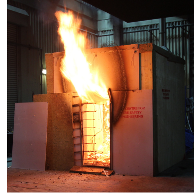
Figure 2.6. Compartment fire experiment on a CLT compartment.
