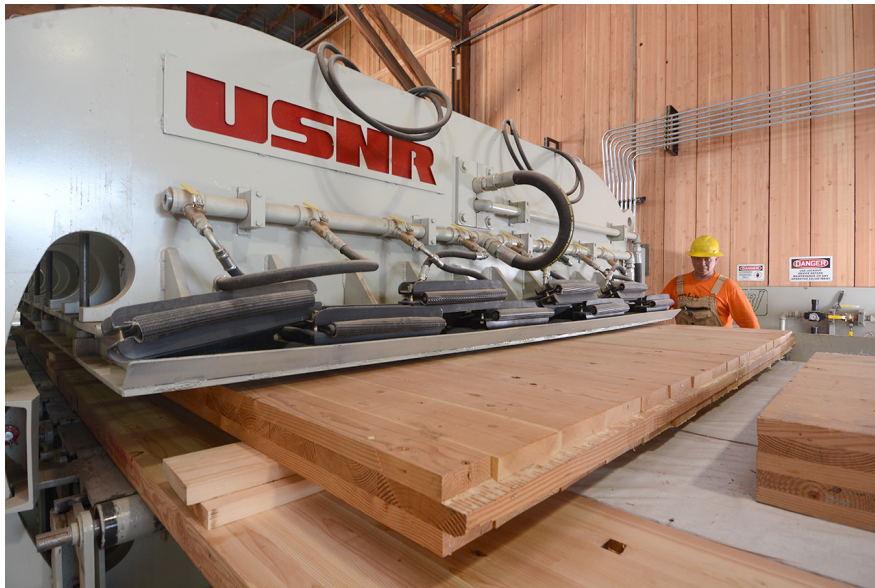
Figure 1.1. Factory production of CLT [4].
