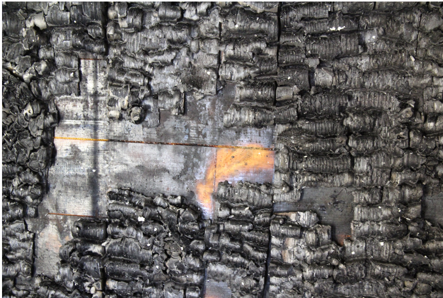
Figure 2.8. Char fall-off (delamination) as observed after a fire in a compartment with polyurethane bonded CLT, from experiments by [129].
