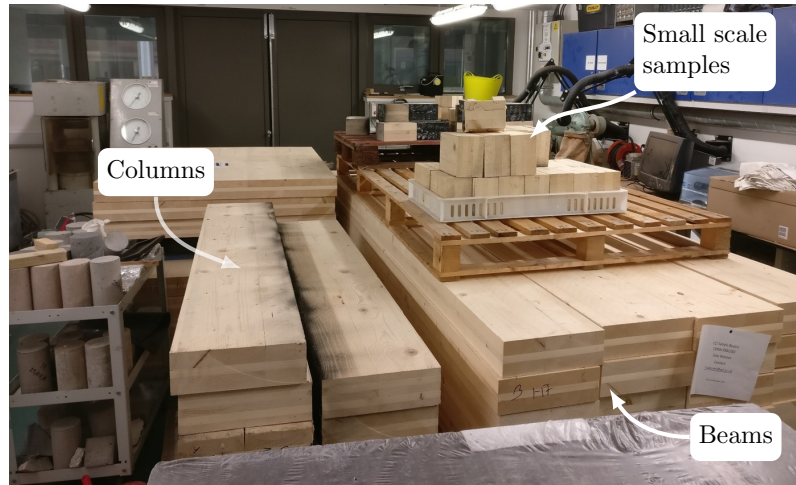
Figure 3.2. Side-by-side comparison of experimental specimen scales in climate controlled storage room.
