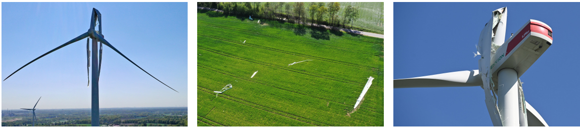
Figure 1.3: Blade Failure. Source: [74]
