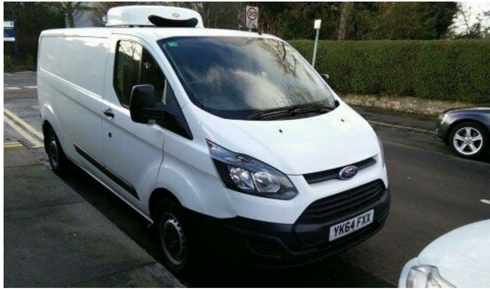
Figure 3.11 - Ford transit custom freezer van. Van was capable of maintaining a temperature of -25^{\circ}\text{C} in the rear compartment.
