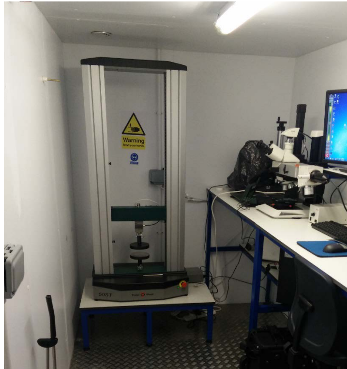
Figure 3.22 - Tinius Olsen 50ST universal tester in place in cold laboratory
