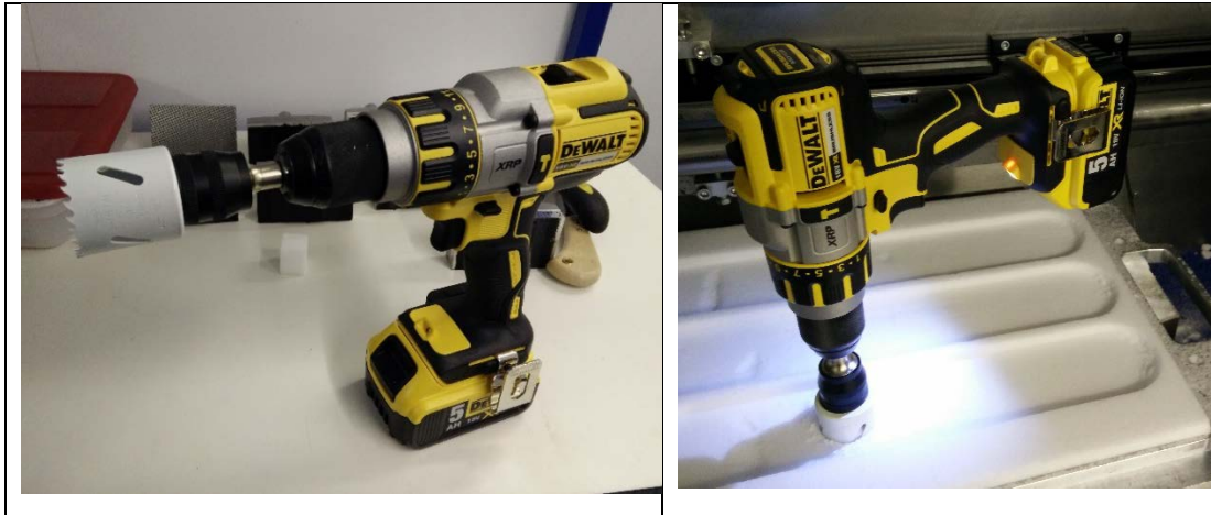
Figure 3.23 - Core drill. Left - bimetal core drill with quick release chuck. Right - Example use of core drill during the development of the testing protocol.
