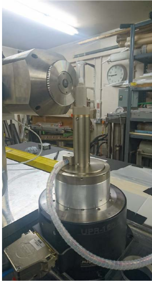
Figure 3.29 - Deben cold stage in place immediately before X-ray scanning. Snow sample can be seen polystyrene chamber.
