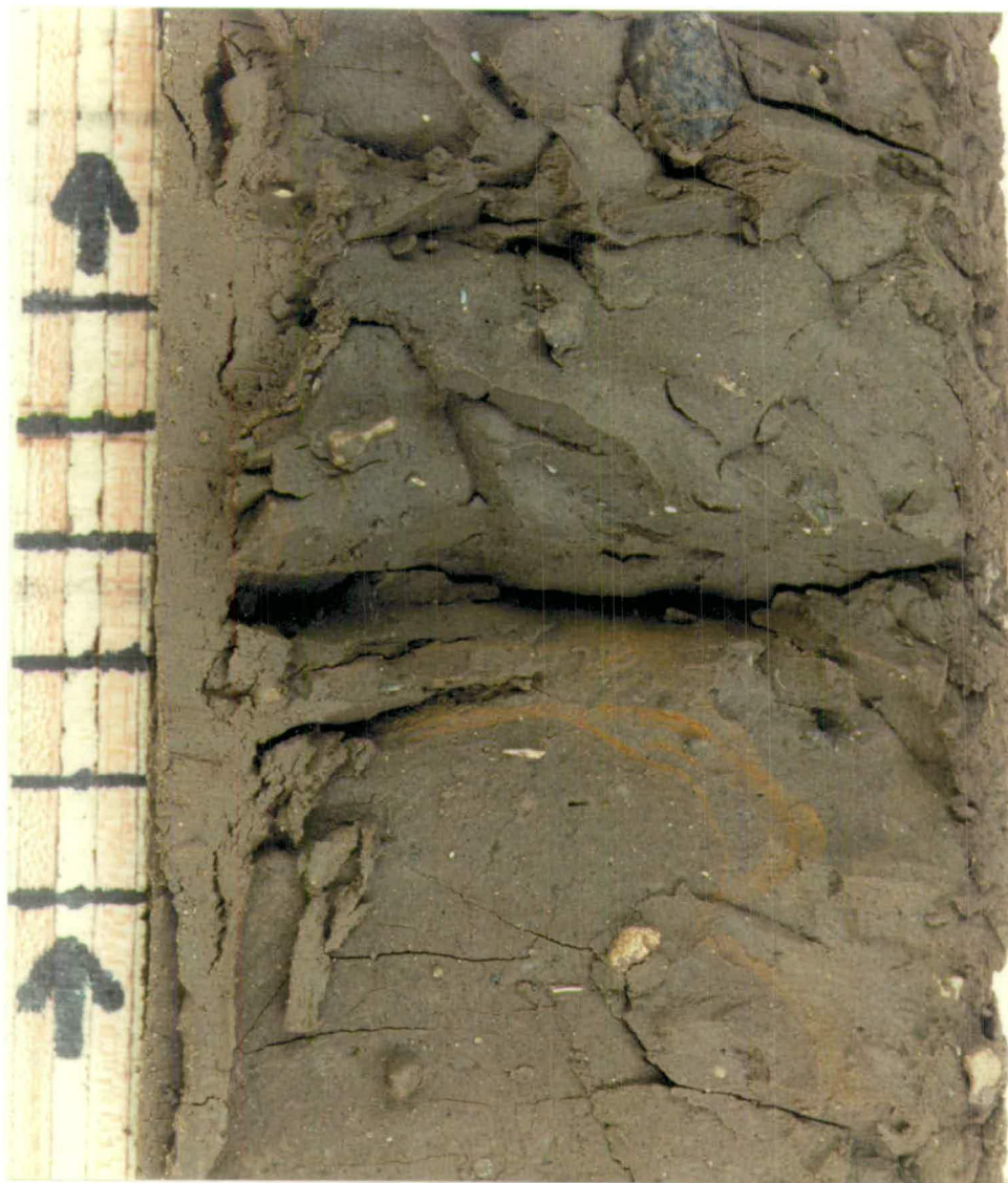
Plates 4.4a. and 4.4b. Facies B 7 , complexly stratified diamict. Note that in places the stratification is highlighted by iron staining. Scale is in centimetres.
