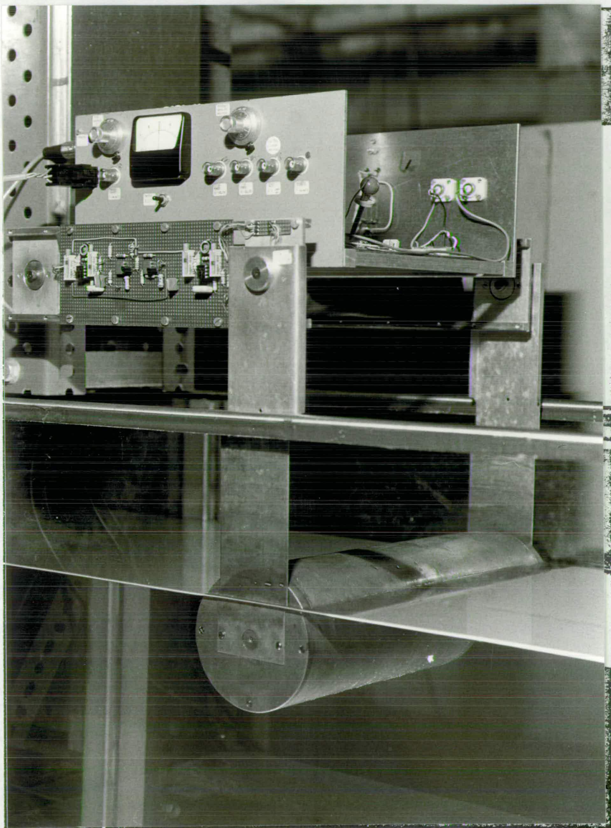
Figure 5.6 The force measuring rig.
