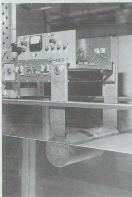
FIG. 10.—Cylinder Mounting and Force Measuring Rig
