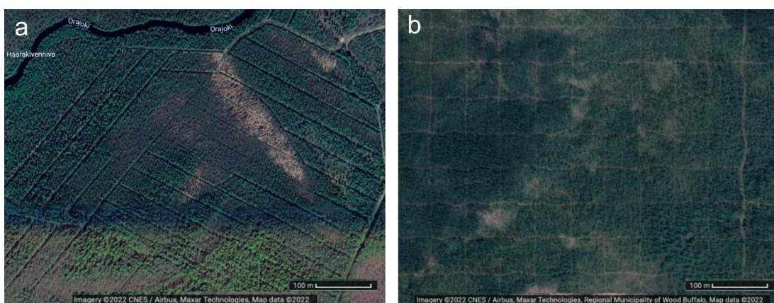
Figure 2.1: Linear features in boreal forest landscapes: (a) Drainage channels used to increase forest productivity in northern Finland; (b) Network of seismic lines for oil and gas exploration in Alberta, Canada. Images are from Google Maps: https://goo.gl/maps/qR9c4Rqj3usX9QvG7 and https://goo.gl/maps/9vLJEcHpsMEbmd8HA respectively.
