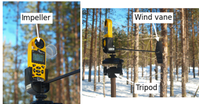
Figure 4.7: A Kestrel 4500 Weather Meter in the field, showing the impeller and weather vane components that are used to measure wind speed and direction, respectively.
