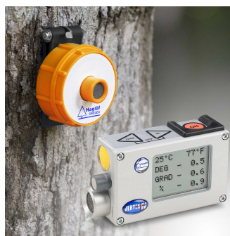
Figure 4.8: The Vertex III Hypsometer and Transponder T3, which were used for measuring tree heights (Haglöf Sweden n.d.)
