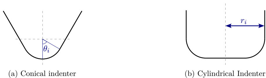
Figure 5.3: Indenters used for the indentation tests. The apex of the conical indenter and the edges of the cylindrical indenter were rounded to a spherical surface with radius 0.005 mm.
