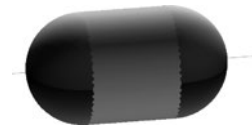
Figure 2.3: A spherocylinder formed using a cylinder and two hemi-spheres, reproduced from Kodam et al. (2010).
