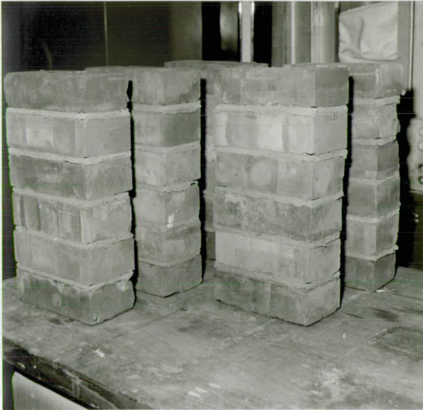
FIG. 7.15 PRISMS READY FOR TEST
