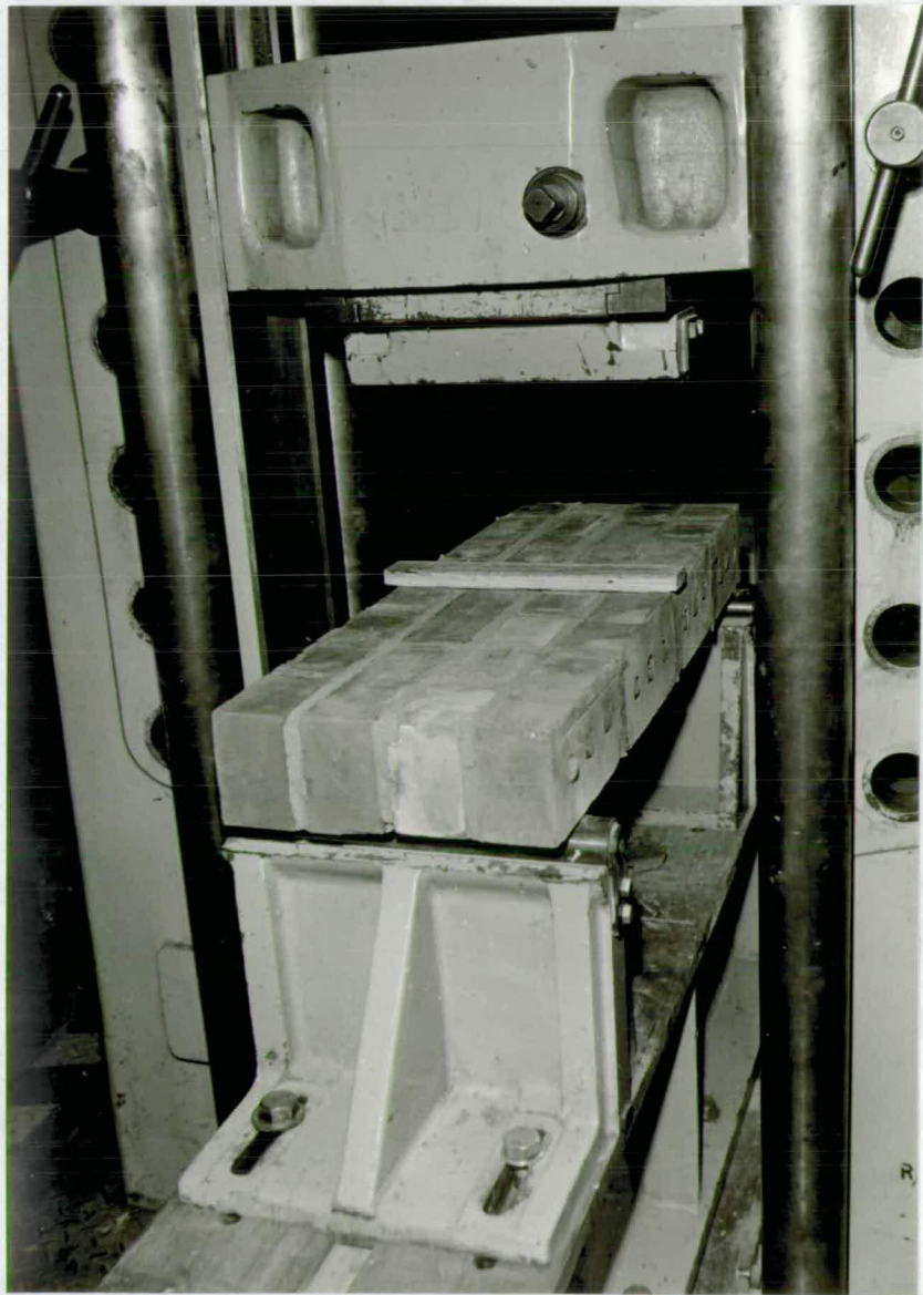
FIG.7.16 WALLETTE PLACED IN TESTING MACHINE
