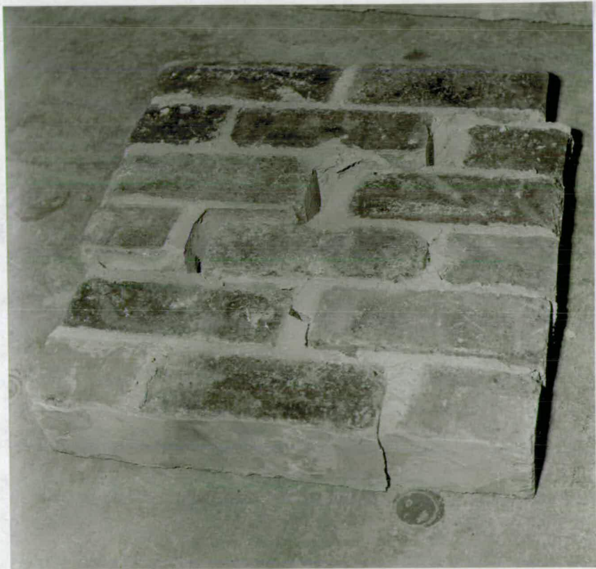
FIG. 7.35 FAILURE OF A WALLETTE OF THE SECOND SERIES
