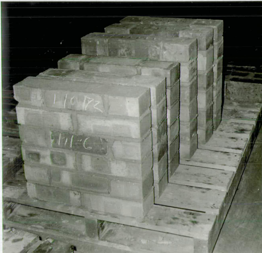
FIG. 7.14 WALLETTES READY FOR TEST
