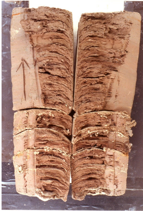
A) Section 24.8 - 25.00m. Well laminated sandy mud facies of Late Devensian age and probable Otterbank sequence affinity.
