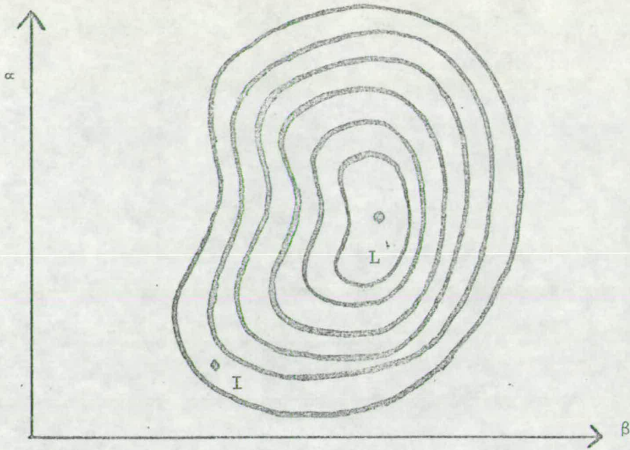
FIGURE 5.8 Error Counter Map for a Non-Linear Problem of Two Variables \alpha, \beta .
