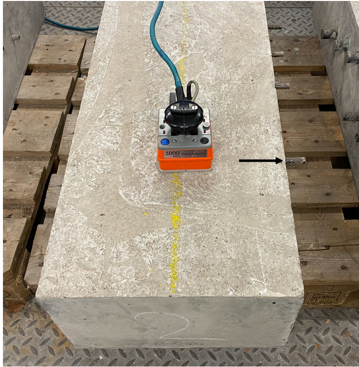
Figure 7.19: Image of the slab for the first case study: 10 traces were selected were selected for FWI from the B-scan taken over the rebar shown with a black arrow.
