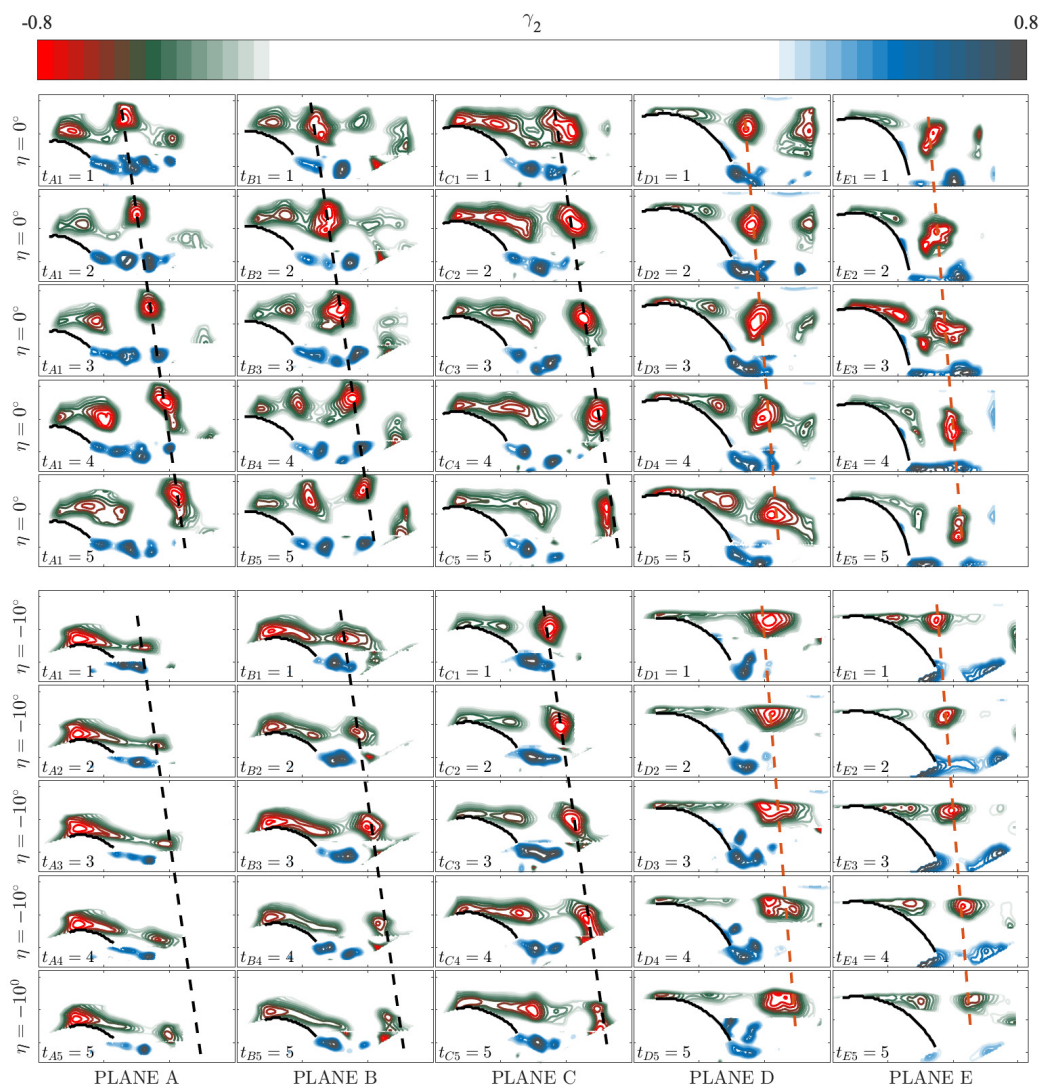
Figure 8.6: Instantaneous sequence of \gamma_2 -contours for planes A, B, C and D of sail S_1 at two incidence angles, \eta = 0^\circ and \eta = -10^\circ
