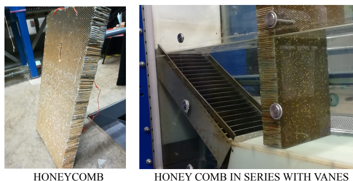
Figure 3.17: Aluminium honeycomb used in series for flow straightening
