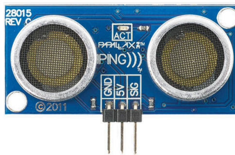
Figure 5-5: Ultrasound sensor (Parallax PING).
