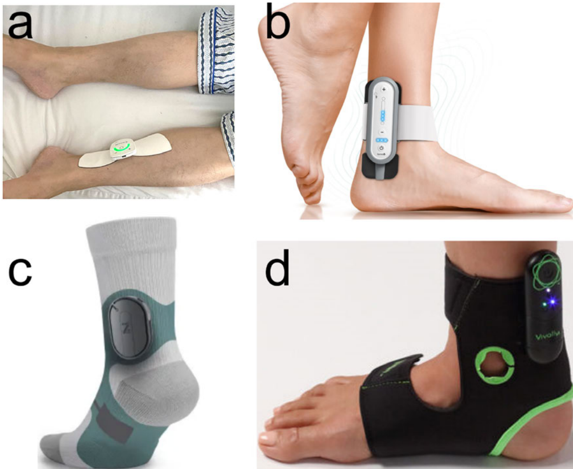
Fig. 2.3. TENS devices used for urinary symptoms (e.g., OAB and UI) management via TTNS: (a) A butterfly-shaped device [103]; (b) TENSi+ device [70]; (c) Zida ® Control Sock [71]; (d) Vivally ® system [72].
