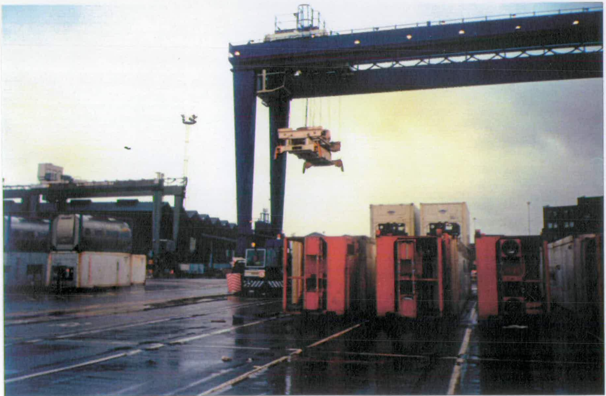
Figure 1.1 A typical Rubber Tyred Gantry (RTG) Crane as used in the container terminals with laden (a.) and unladen (b.) spreader
