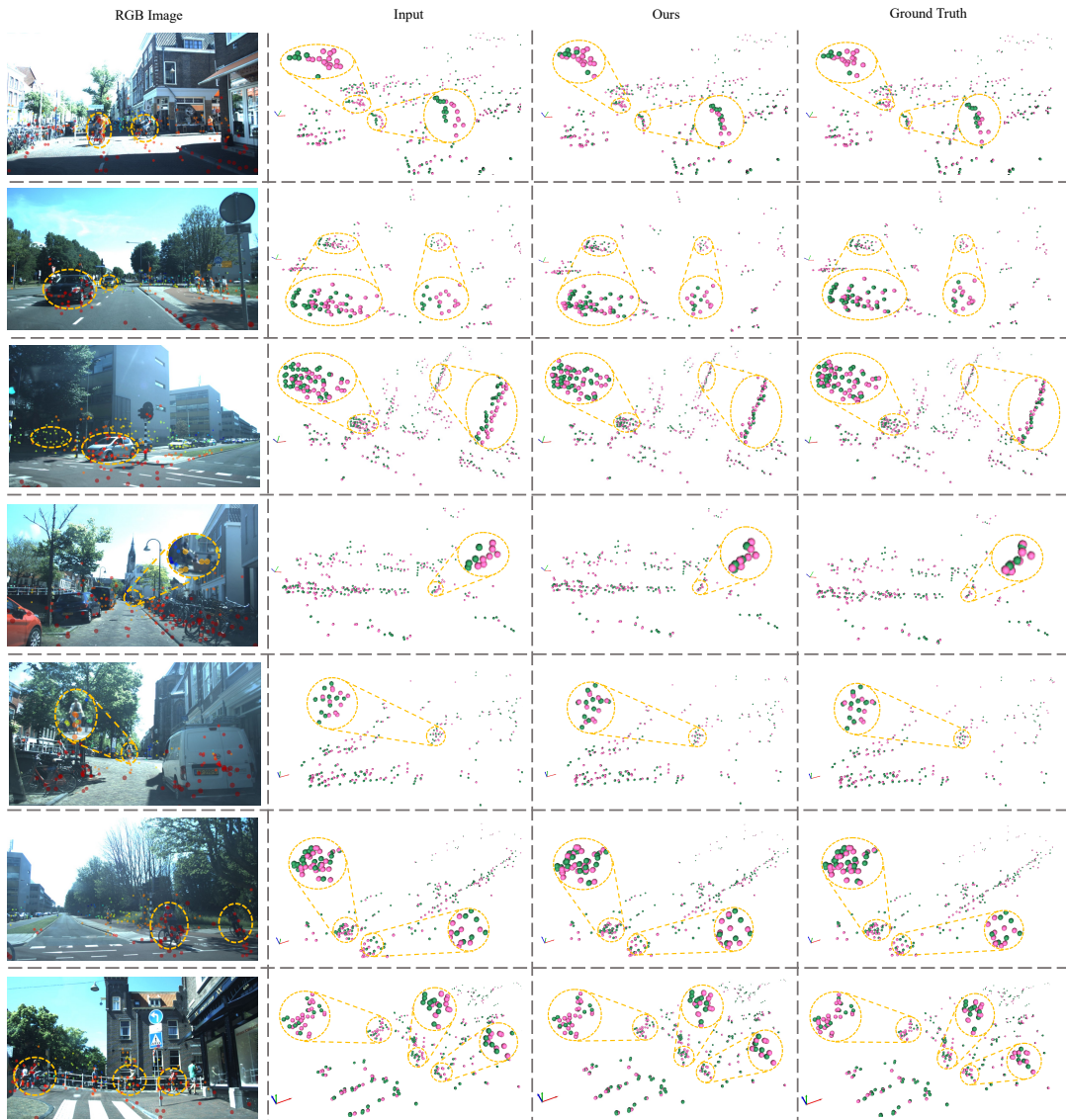
Figure A.5: Qualitative scene flow results in seven Test scenes. From left to right: 1) radar points from the source frame projected to the corresponding RGB image (points are coloured by distance from the sensor), 2) two input radar point clouds, the source one (pink) and the target one (green), 3) the source point cloud warped by our predicted scene flow and the target radar point cloud, 4) the source point cloud warped by ground truth scene flow and the target one. We mark regions of interest in amber and apply the zooming-in operation for them.
