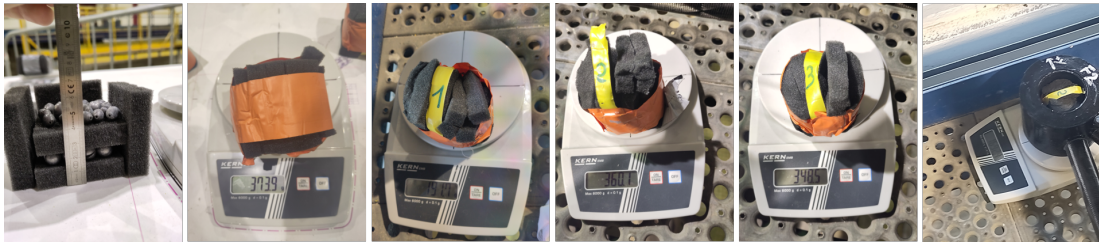
Figure 6.18: View of ballast weights preparation
