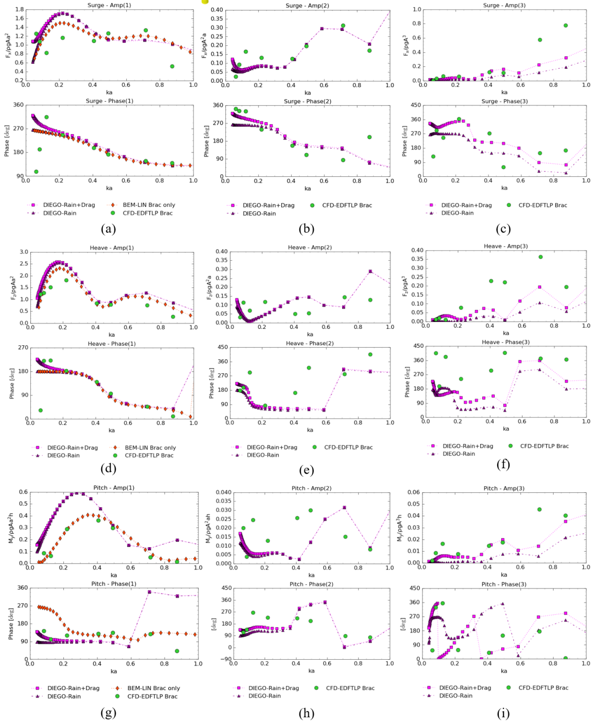
Figure 5.13: Comparison of normalised first, second and third-order surge (a)(b)(c), heave force (d)(e)(f) and pitch moment (g)(h)(i) transfer functions on the bracings of the EDF-TLP
