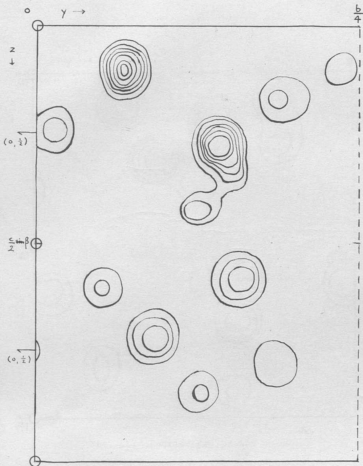
Fig. 10. Fourier projection on 100. (Contours at 10, 15...40 electrons/ \text{\AA}^2 .)
