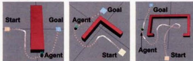
Figure 4.18: Escaping from bench, corner and dead-end.
