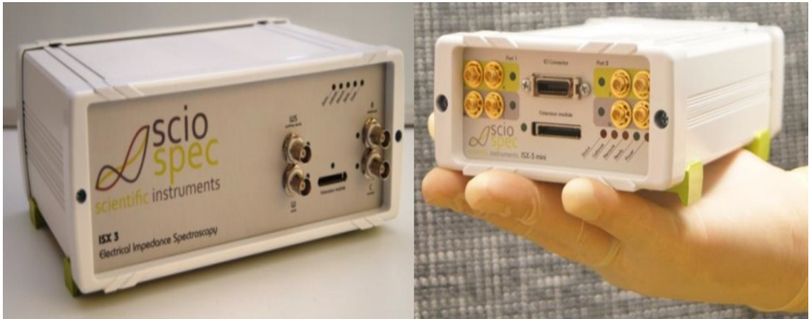
Figure 3-5 Sciospec ISX-3v2 electrical impedance spectroscopy [16].
